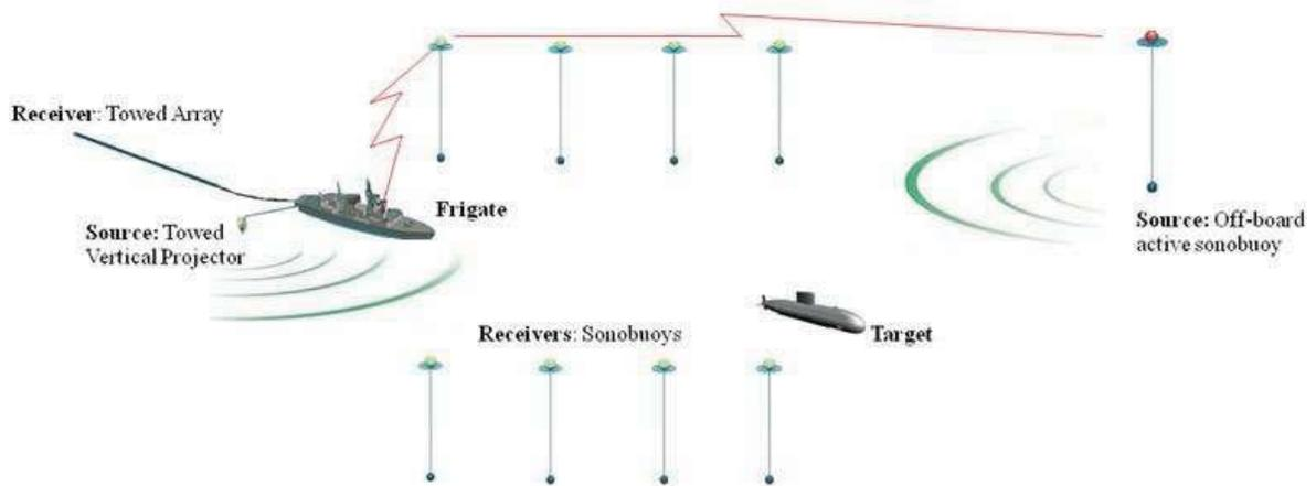
(c) Same as 3(a) except multiple sources may also be deployed such as the frigate's HMS.
