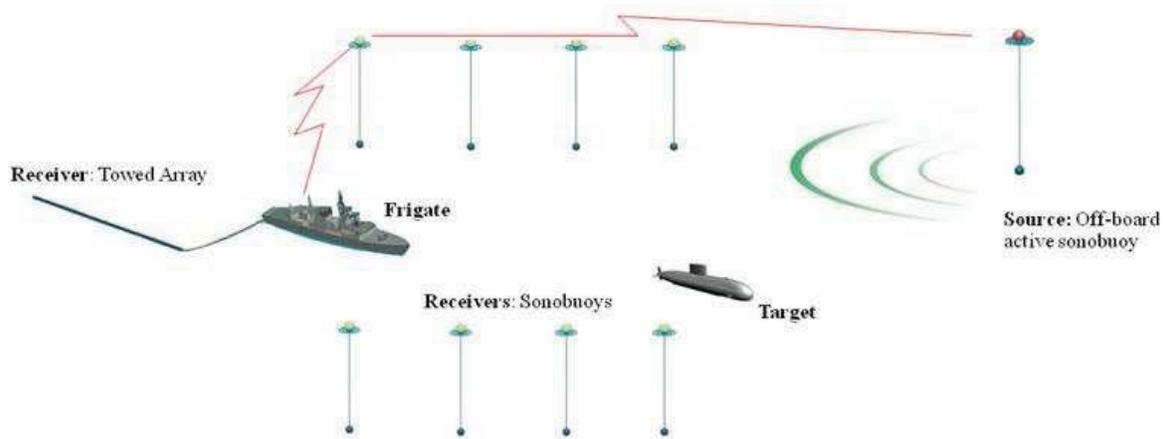
(b) Same as 3(a) except multiple sources may be deployed such as a towed vertical projector from a frigate.
