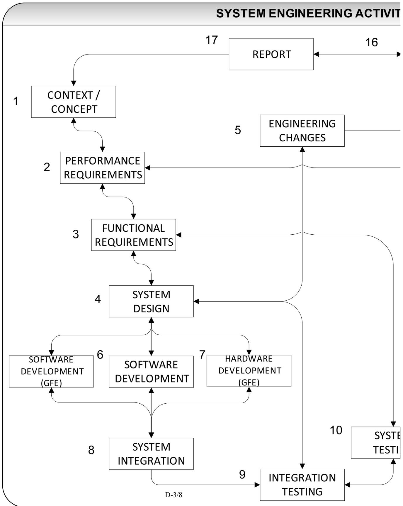
*Figure 1. Proposed system engineering process for the development and trial phases. This is a simplified process diagram and the activities will interact with each other in ways not shown, and will be tailored to the specific needs of a project phase.*
