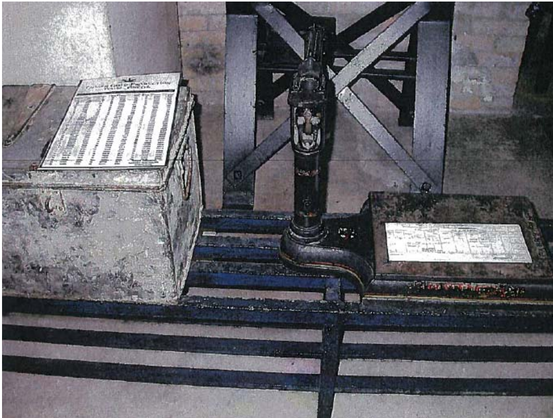
Photo 35: Rack and balance beam scale beside furnace
