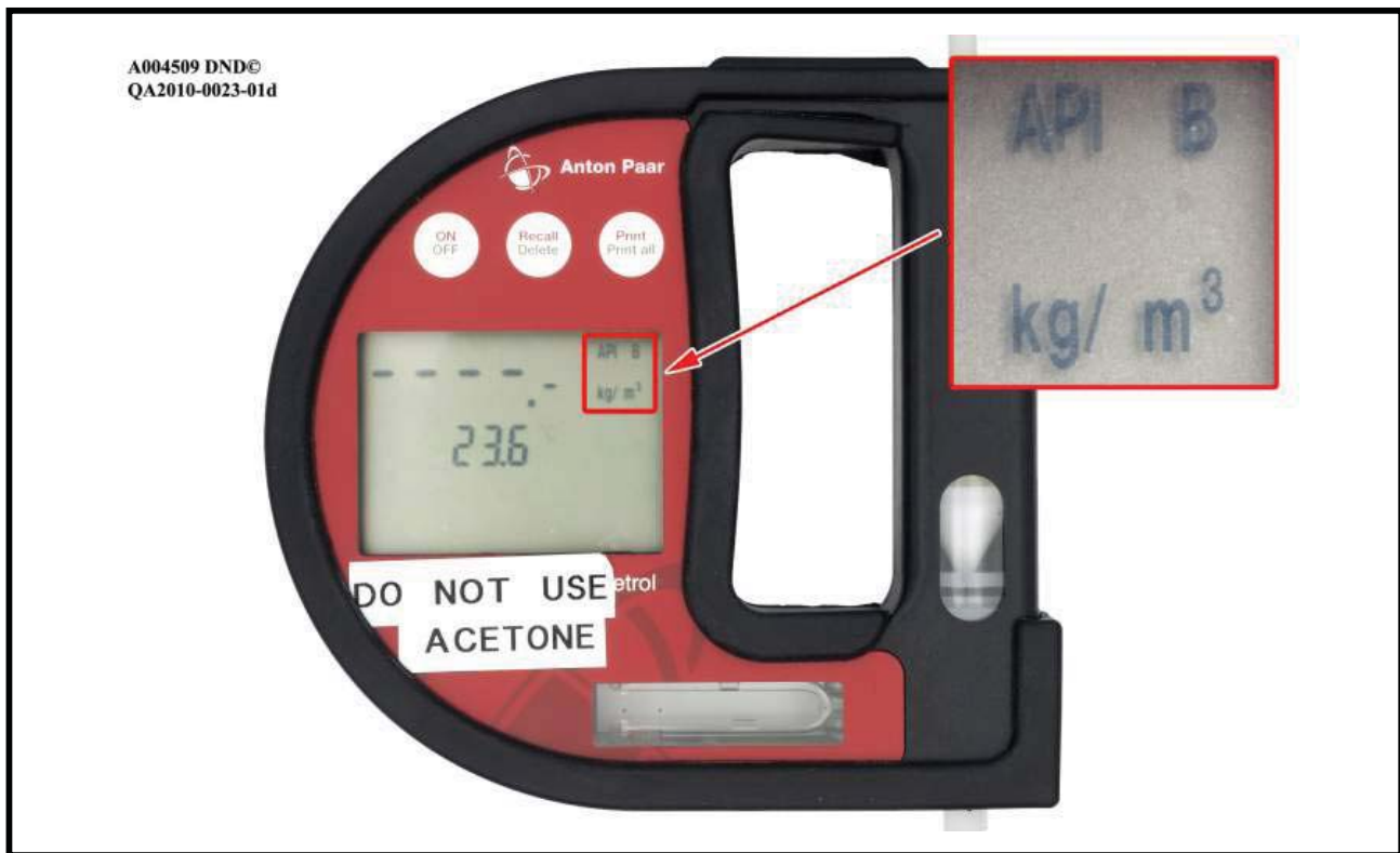
Figure G-1 DMA 35N Portable Density Meter Figure G-1 Densimètre portatif DMA 35N
