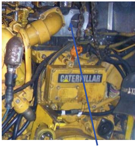
E-02-2 Typical Aftercooler
