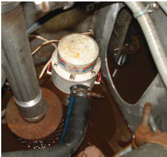
Engine Room Submersible pump port E-12-02
