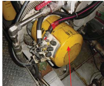
Figure L-01-3 Port alternator
