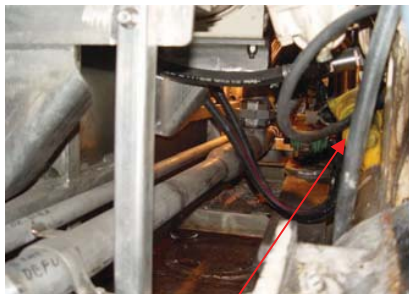
Figure L-01-2 Port starter
