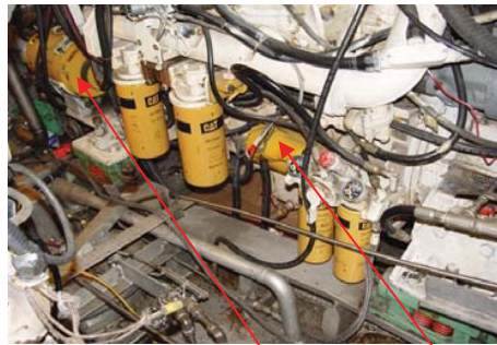
Figure L-01-1 Starboard alternator and starter
