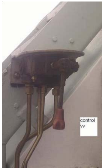
Control valve for the capstan hauler
