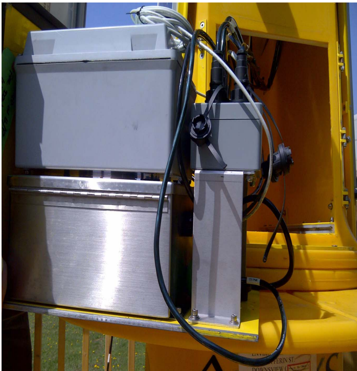
Figure 5 – 1.7M Watchkeeper Buoy- Payload Assembly
