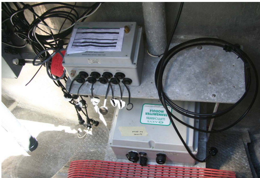
Figure 31 – 6M Nomad Buoy- Payload and Transmitter Top View
