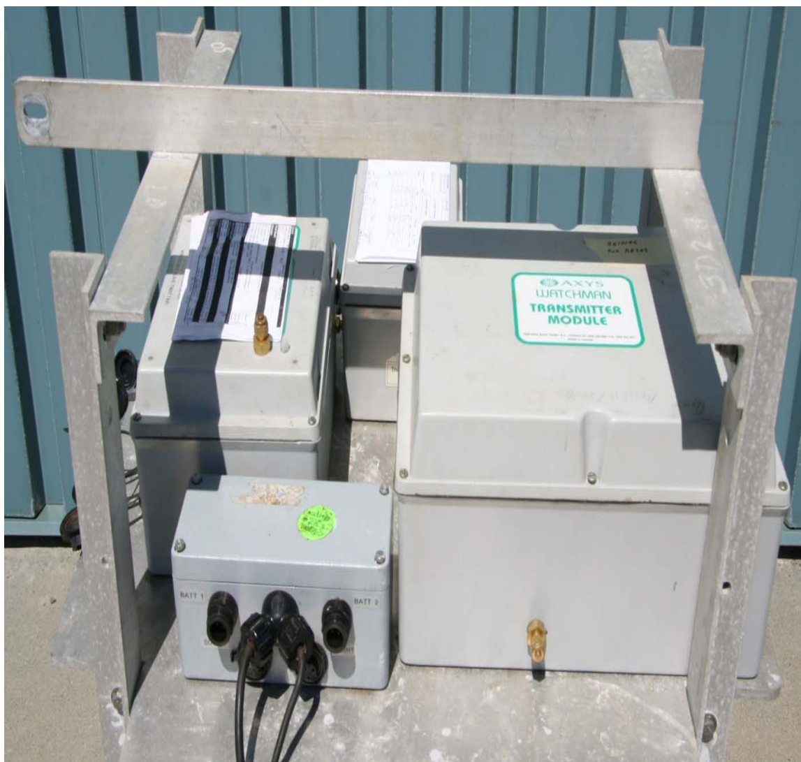
Figure 8 – 3M Discus Buoy- Payload Shelf
