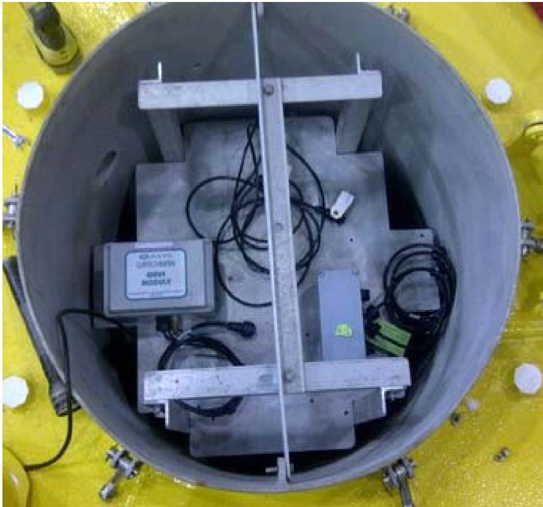
Figure 9 – 3M Discus Buoy- Hull Well Top View
