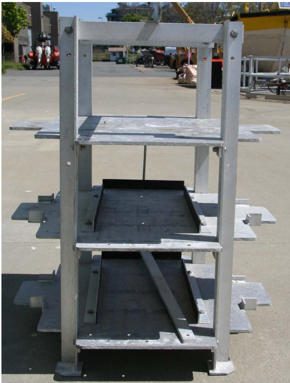
Figure 7 – 3M Buoy Discus - Battery and Payload Rack
