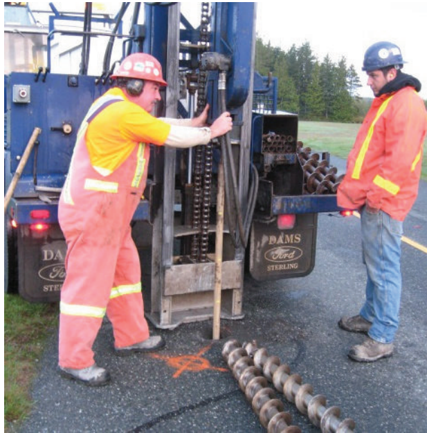
Photo 1: Conducting DCPT at AH10-03.
