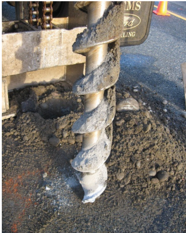
Photo 2: Practical refusal of solid stem auger hole at AH10-03. Cobbles pulverized by drilling (light grey) shown on auger flights.
