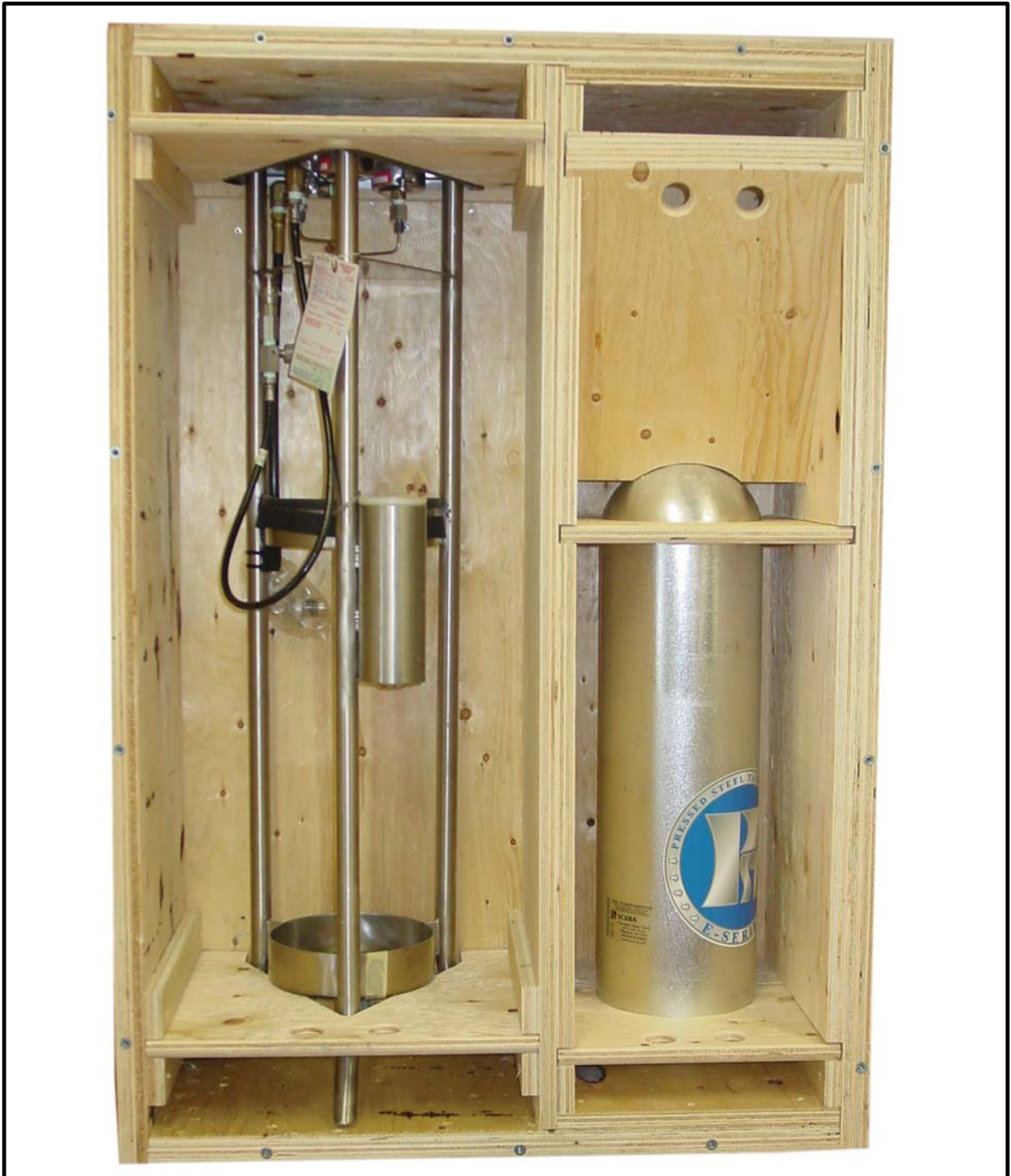
Figure 4-4 PRS Packed in Shipping Crate and Braced
