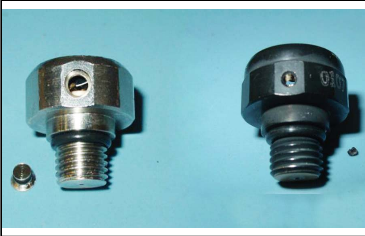
Figure 2-1-1 Pressure Gauge Blow-out Disc
