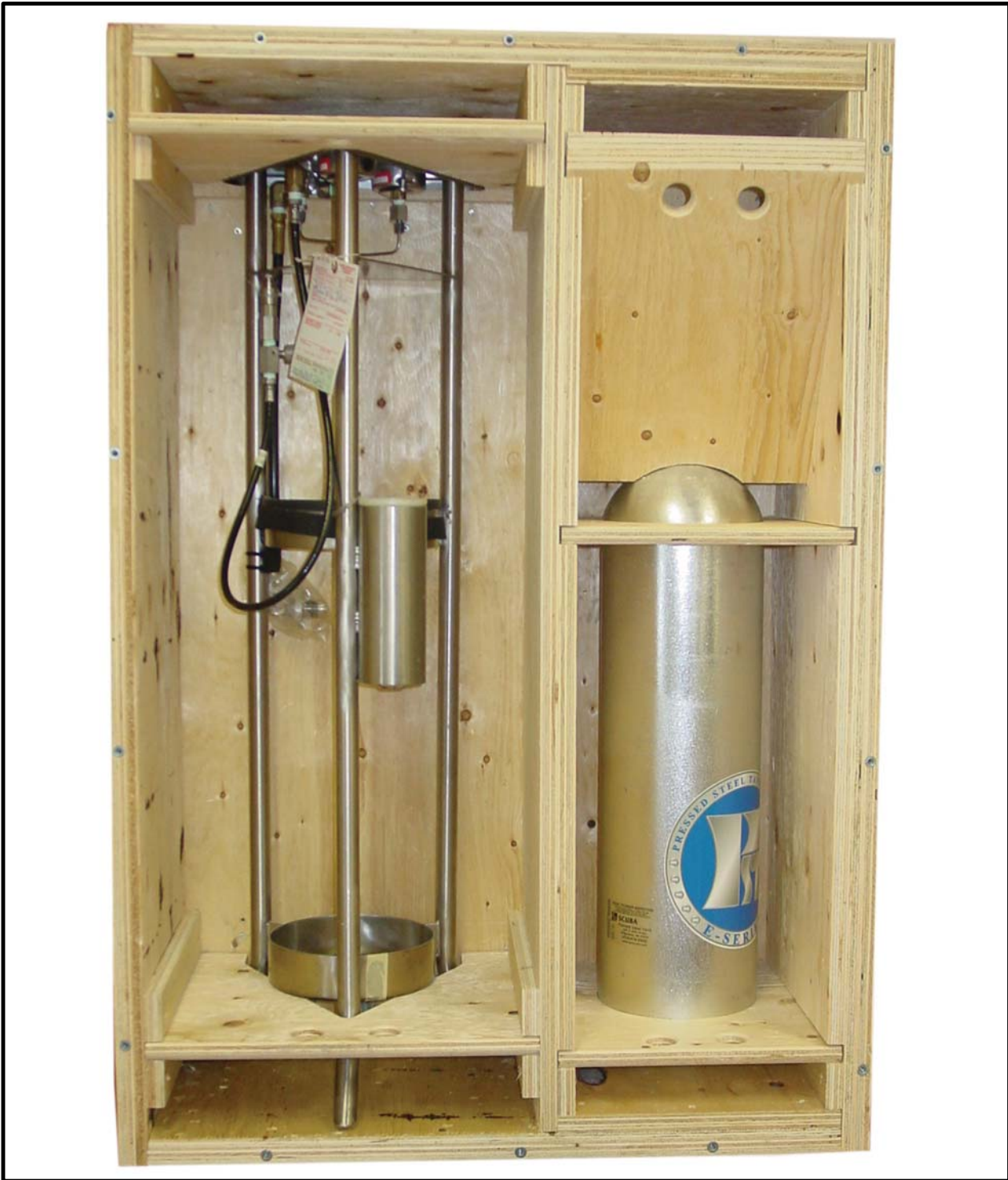
Figure 5-1-4 PRS Packed in Reusable Shipping Crate and Braced
