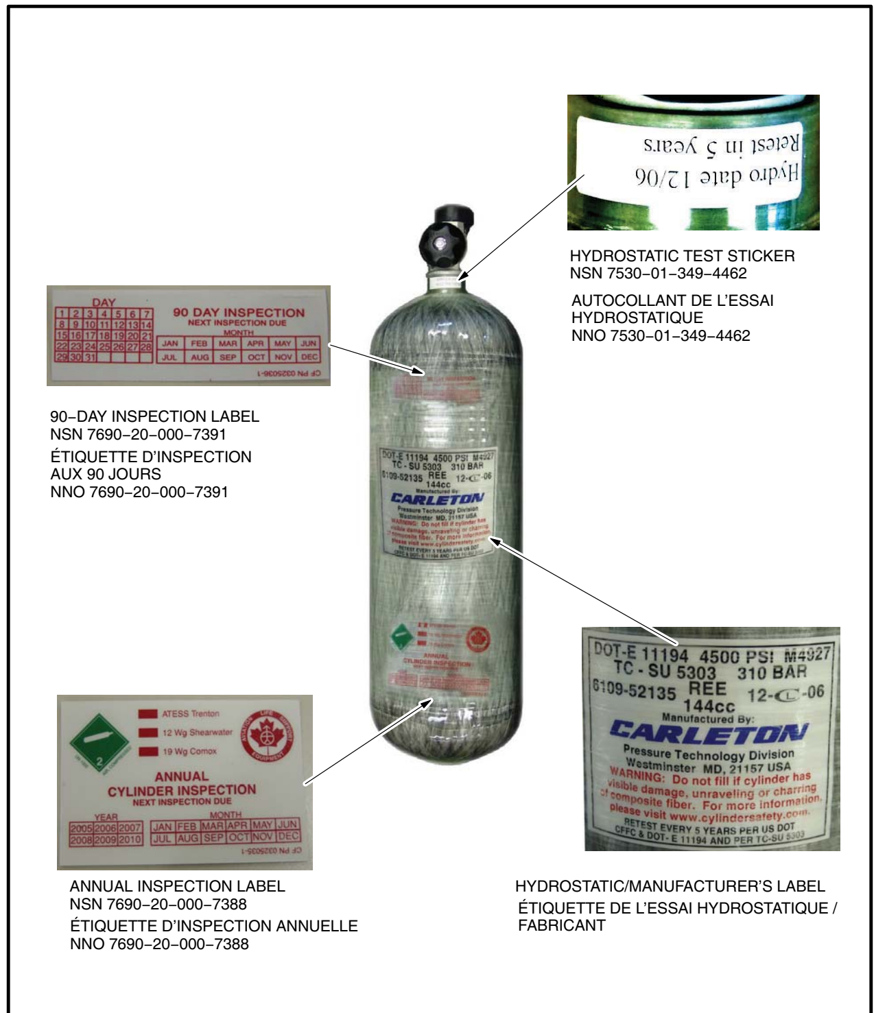
Figure 3-1-2 Various Labels Required for MRS Cylinder
