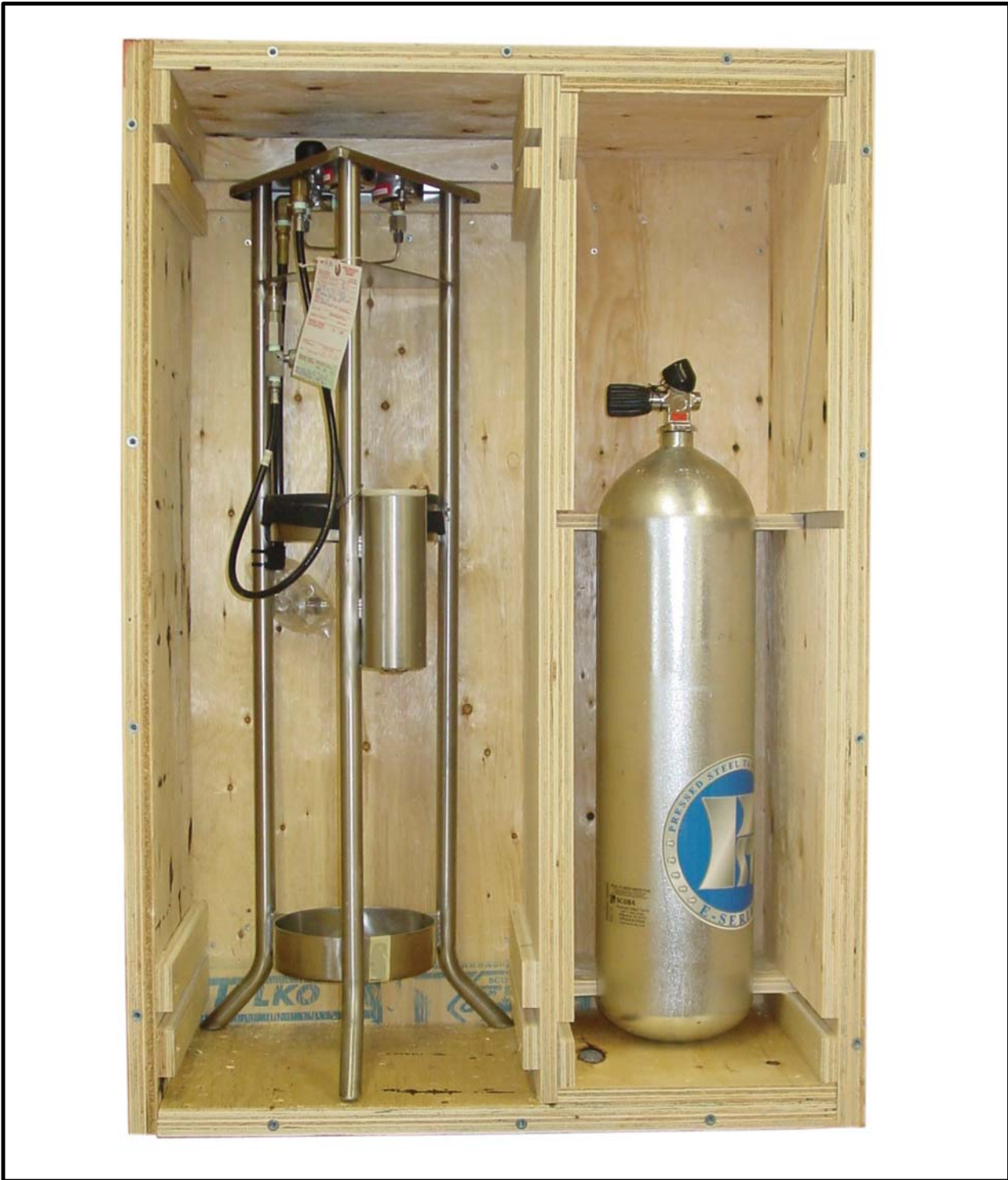
Figure 4-3 PRS Positioned in Shipping Crate
