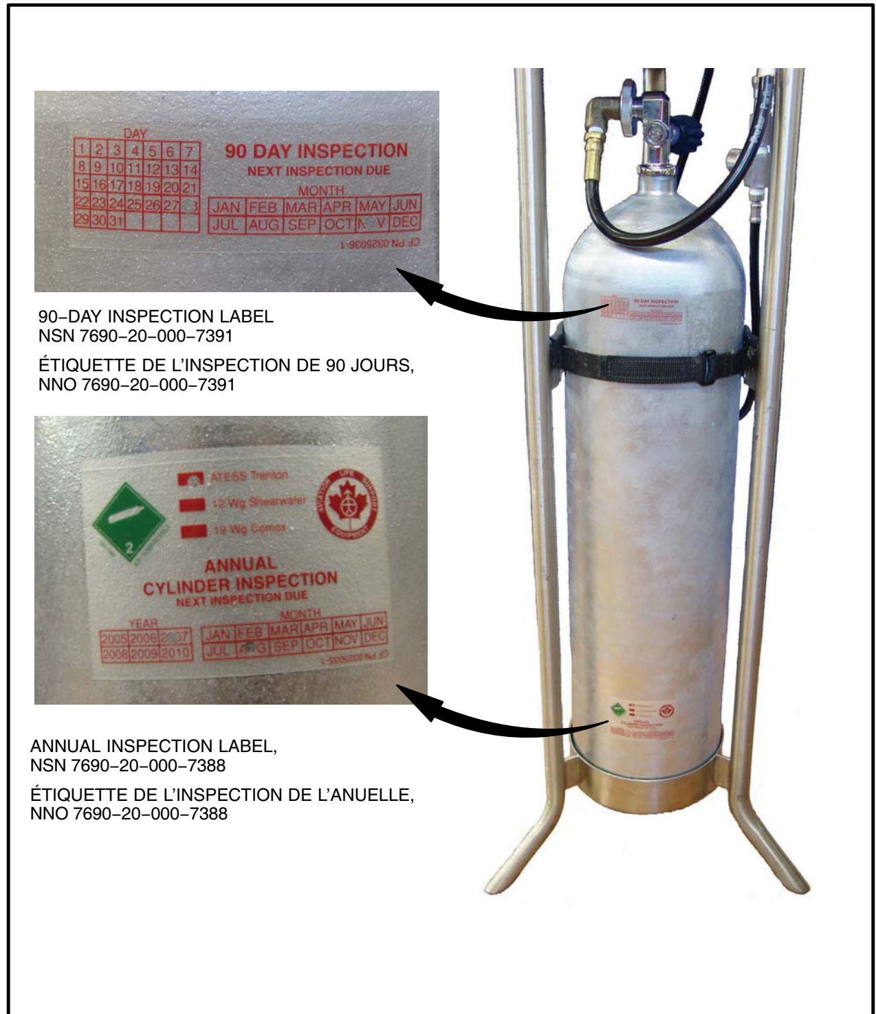
Figure 3-1-3 Orientation of 90-day and Annual Inspection Labels
