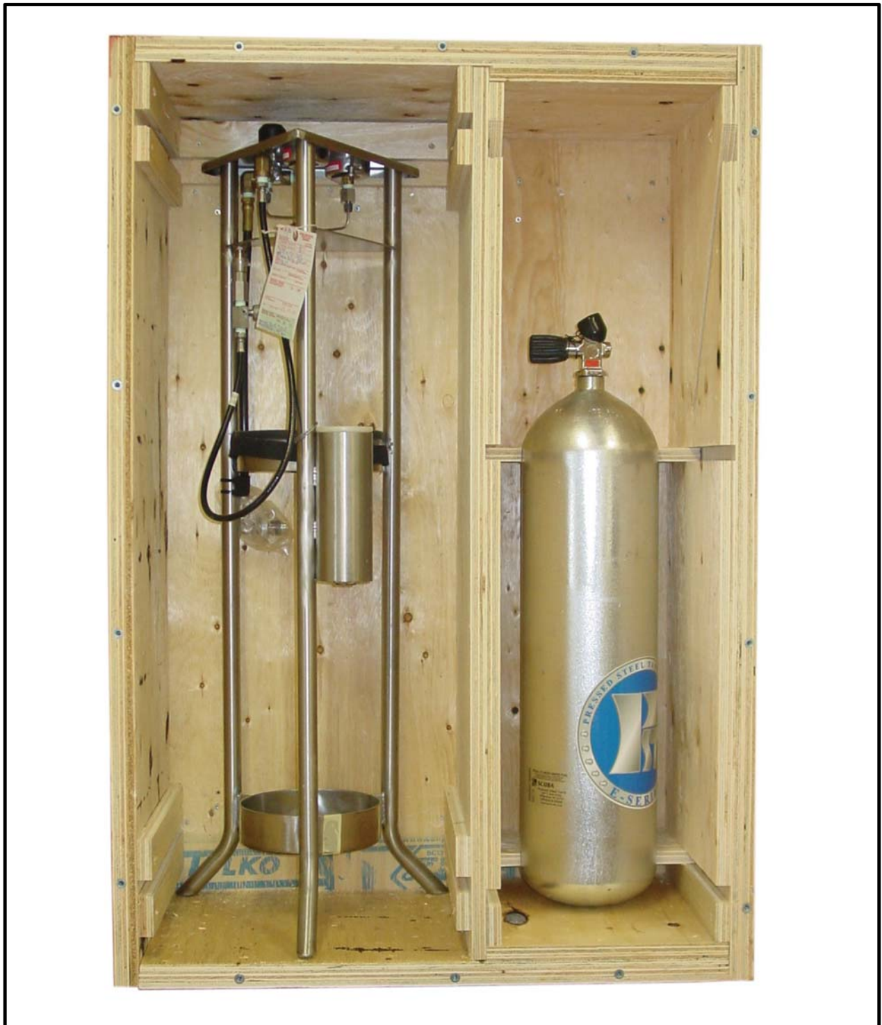
Figure 5-1-3 PRS Positioned in Reusable Shipping Crate
