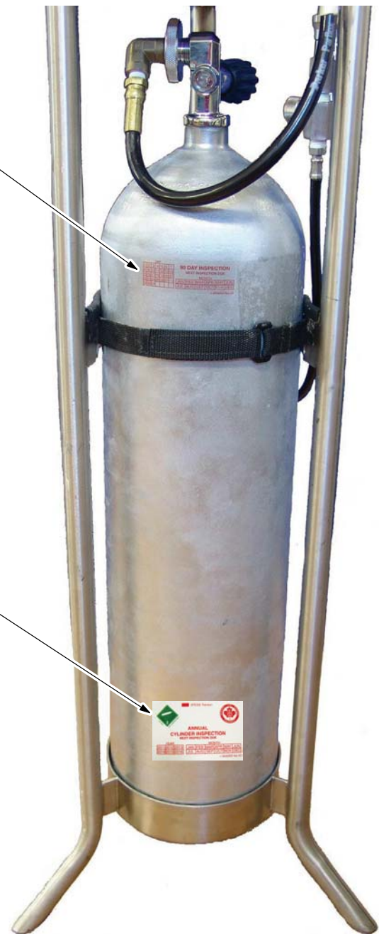
Figure 2-1-3 Orientation of 90 day and Annual Cylinder Inspection Labels
