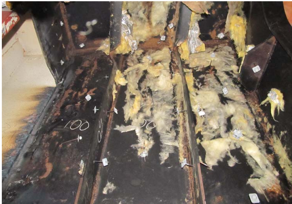
Damaged frames, brackets forward of bulkhead at frame 35
