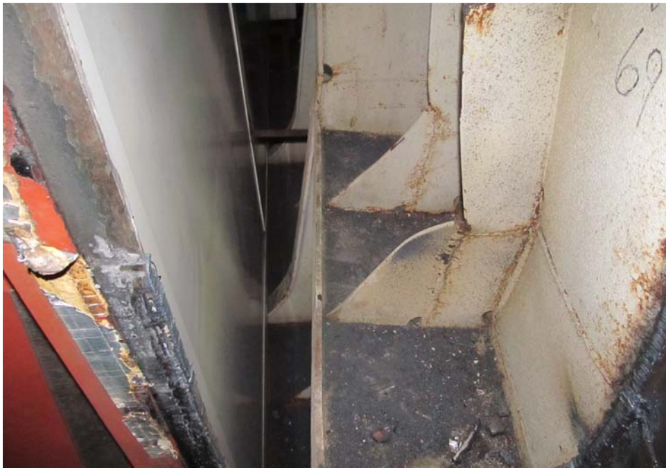
Damaged frames, brackets aft of bulkhead
