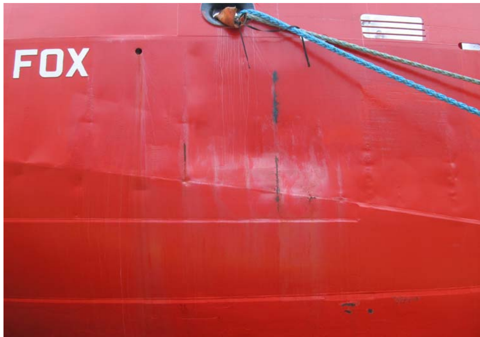
Port Side Damage - Exterior View
