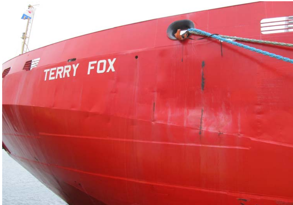
Port Side Damage - Exterior View
