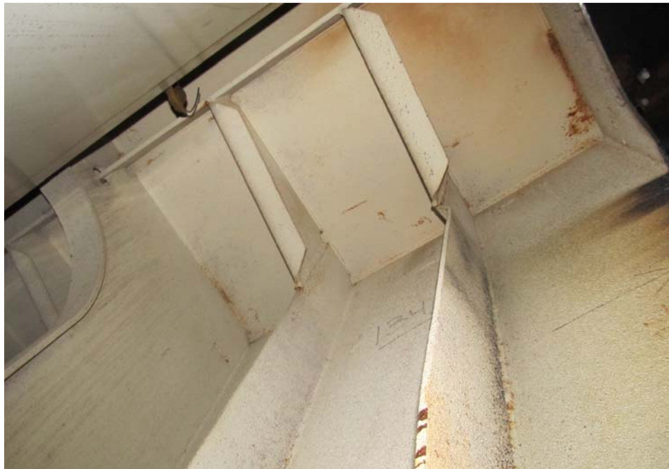
Damaged frames, brackets aft of bulkhead
