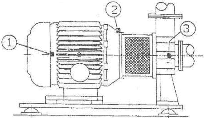
Block 1: On motor non-drive end housing, front side (when facing the terminal box cover), on boss 2 inches above cooling ribs.
