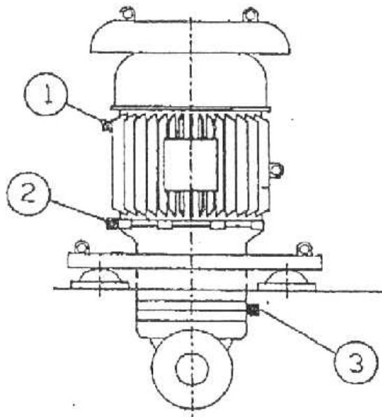
Block 1: On motor body/frame, left side (when facing terminal box cover), 1 in below fan hood.
