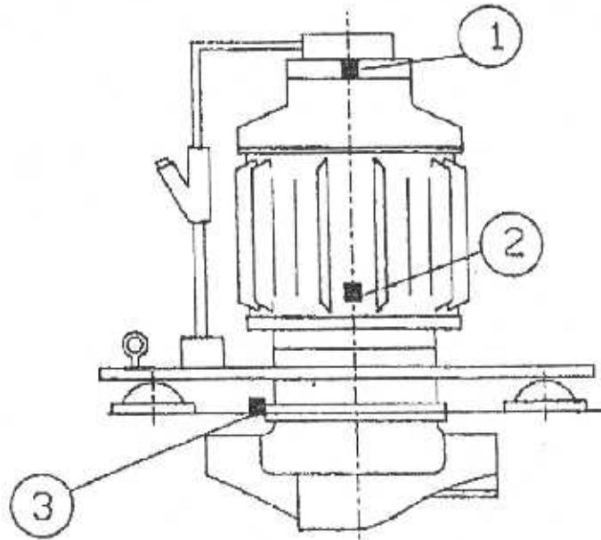
Block 1: On motor non-drive end, top flange, back side (when facing the terminal box cover)
