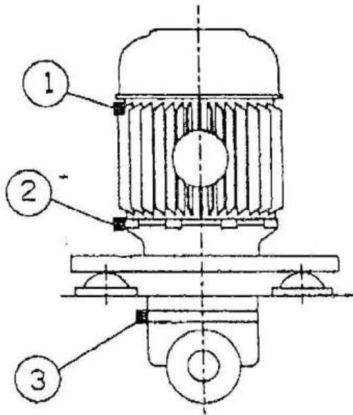
Vibration block locations are as indicated on the attached drawing.
