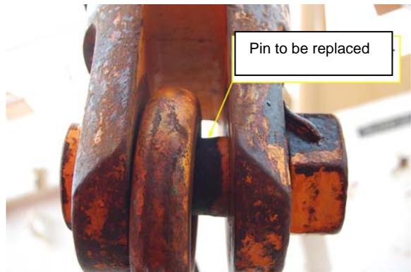
7. Check the side play of pulleys #7 (8 tons) and #20 (5 tons) that seems excessive. Check the grease ways, measure and check the wear of all parts. Carry a load test and supply a load test certificate. Replacement parts will be extra work.
