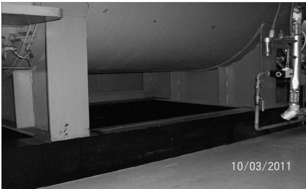
Side view showing existing autoclave mounting structure welded to I-beams.
