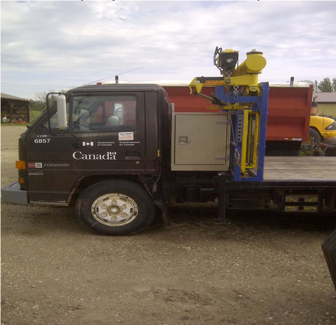
Photo #1 - Current set-up, existing crane and tool box to be installed on new platform.
