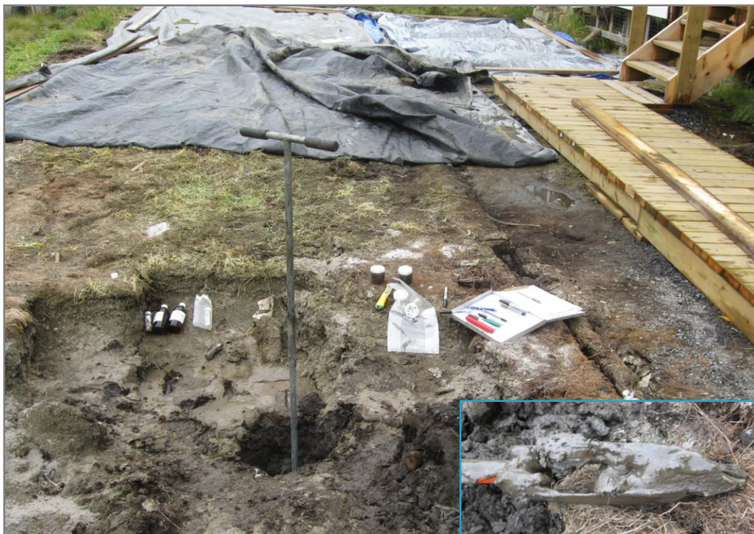
Photograph 8. TH11-02 location; view facing west over south end of house. PHC sheen on soil at depth of water (inset). ↑
