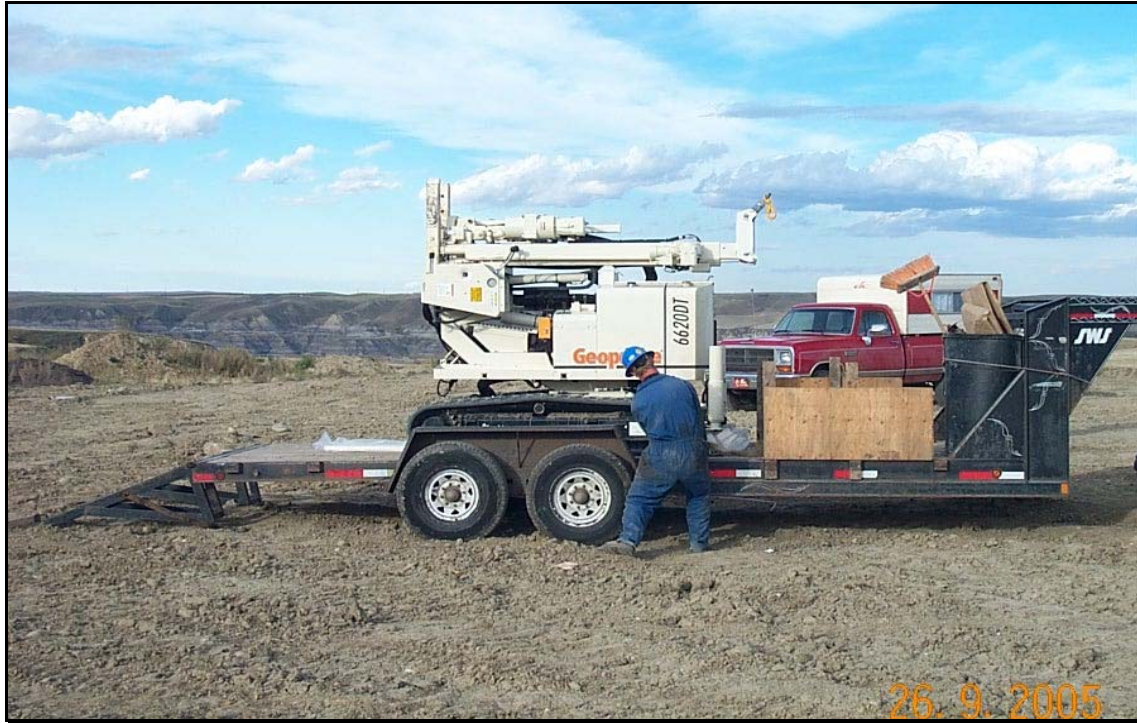
Photograph 9 - Truck-mounted direct push unit used for borehole drilling.
