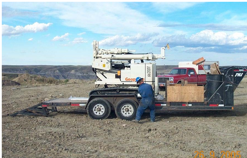
Photograph 6: Truck-mounted direct push unit used for drilling of boreholes.
