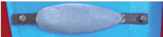
Figure HD-04-3 Rudder anode
