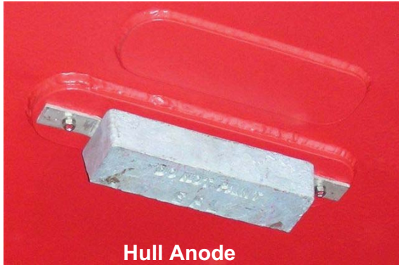
Figure HD-04-1 (10) Kg Zinc Hull / Transom anodes
