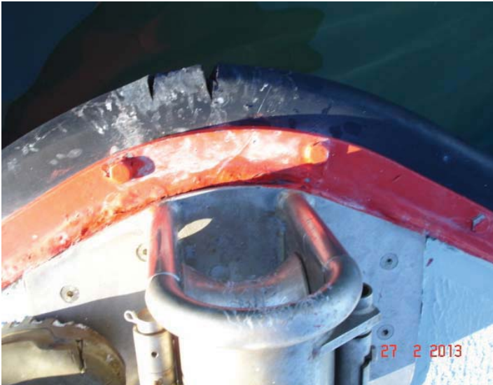
HD-01-1 Damaged area of D Rubber
