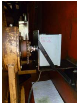
Encoder installed on the CCGS Amundsen
