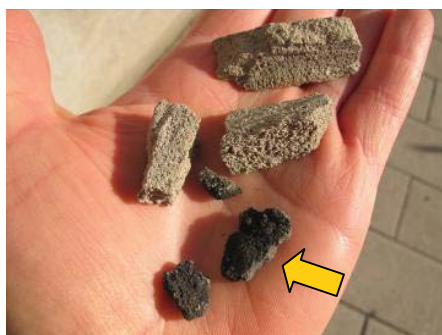
Figure 15 Black mortar scraps collected behind the more recent grey joints of the ground floor granite cladding.
