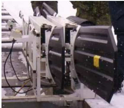
Figure 3- Original OEM targets mounted on ATS lifter
