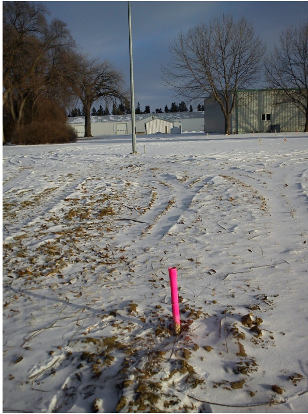
Photo 3 - Standpipe piezometer installed in Testhole TH 04
