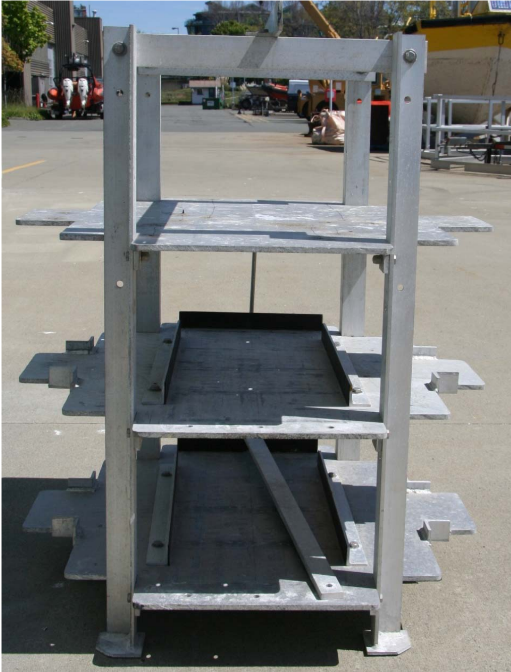
Figure 7 – 3M Buoy Discus - Battery and Payload Rack
