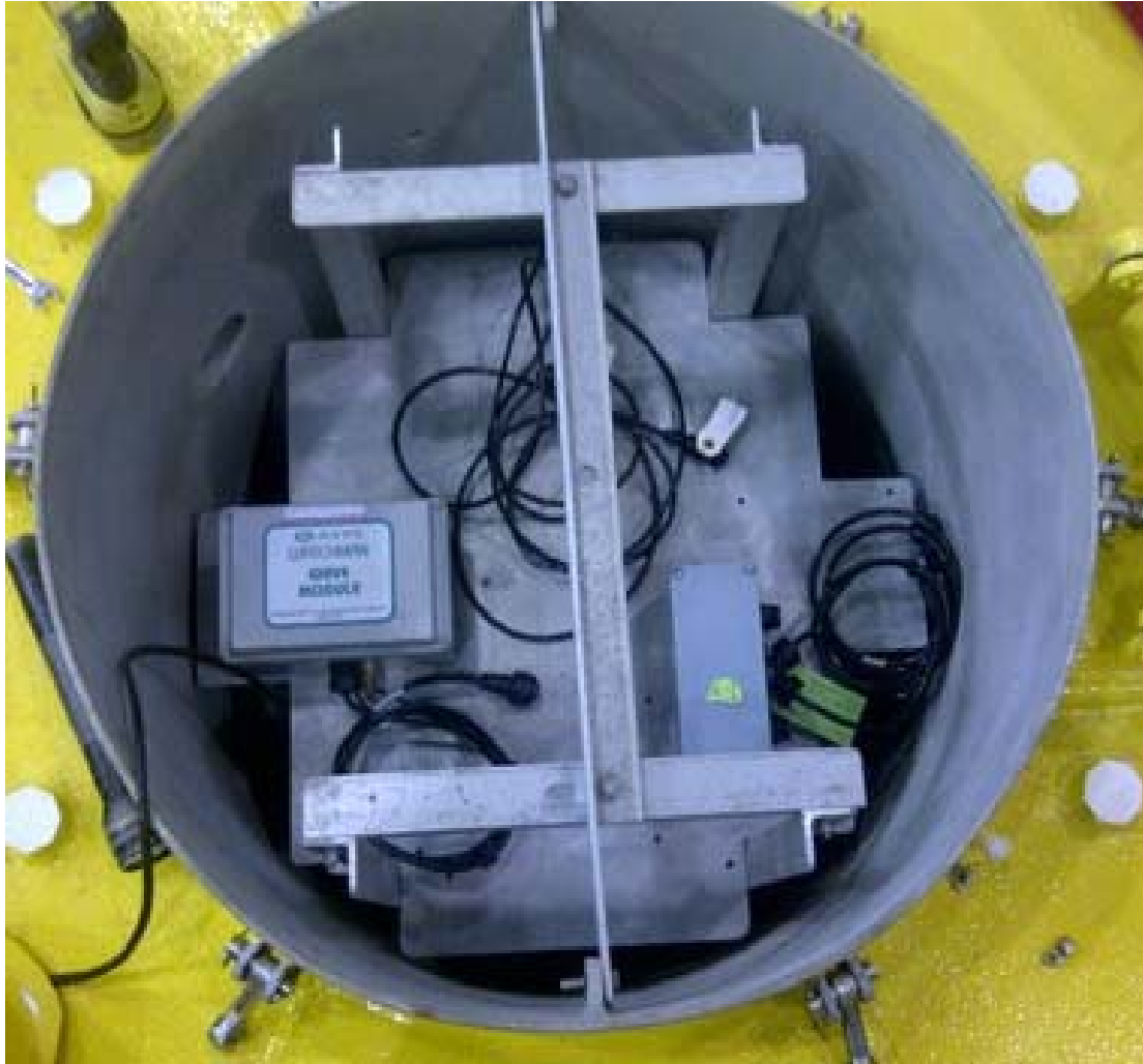
Figure 9 – 3M Discus Buoy- Hull Well Top View
