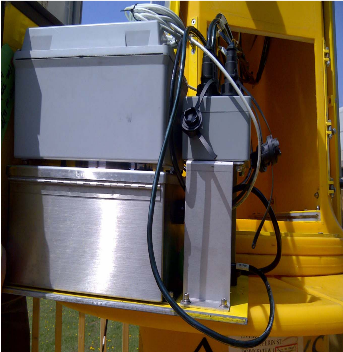
Figure 5 – 1.7M Watchkeeper Buoy- Payload Assembly
