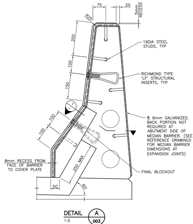
16mm DIA TYPE 304 STAINLESS STEEL HEXAGONAL HEAD BOLT COUNTERSUNK INTO 50 mm DIA RECESS. INSTALL USING "KOP-R-KOTE" OR "NEVER SEEZ" ON THREADS AND UNDER HEADS. SNUG TIGHTEN BOLTS IN SHOP FOR TRANSPORTATION
