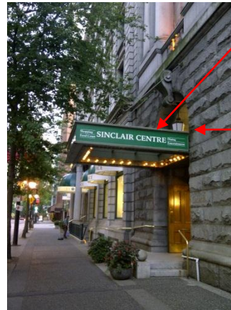
P2. DEMOLISH EXISTING CANOPY REMOVE EX. LIGHT FIXTURE (REFER TO ELEC.)
