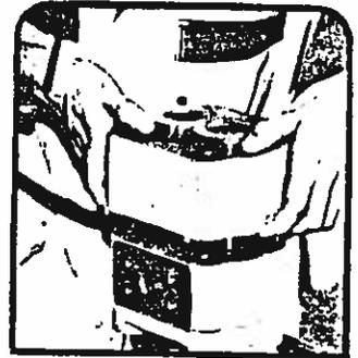
Lift or pry off the bearing carrier carefully to prevent damage to contact face and edges.
