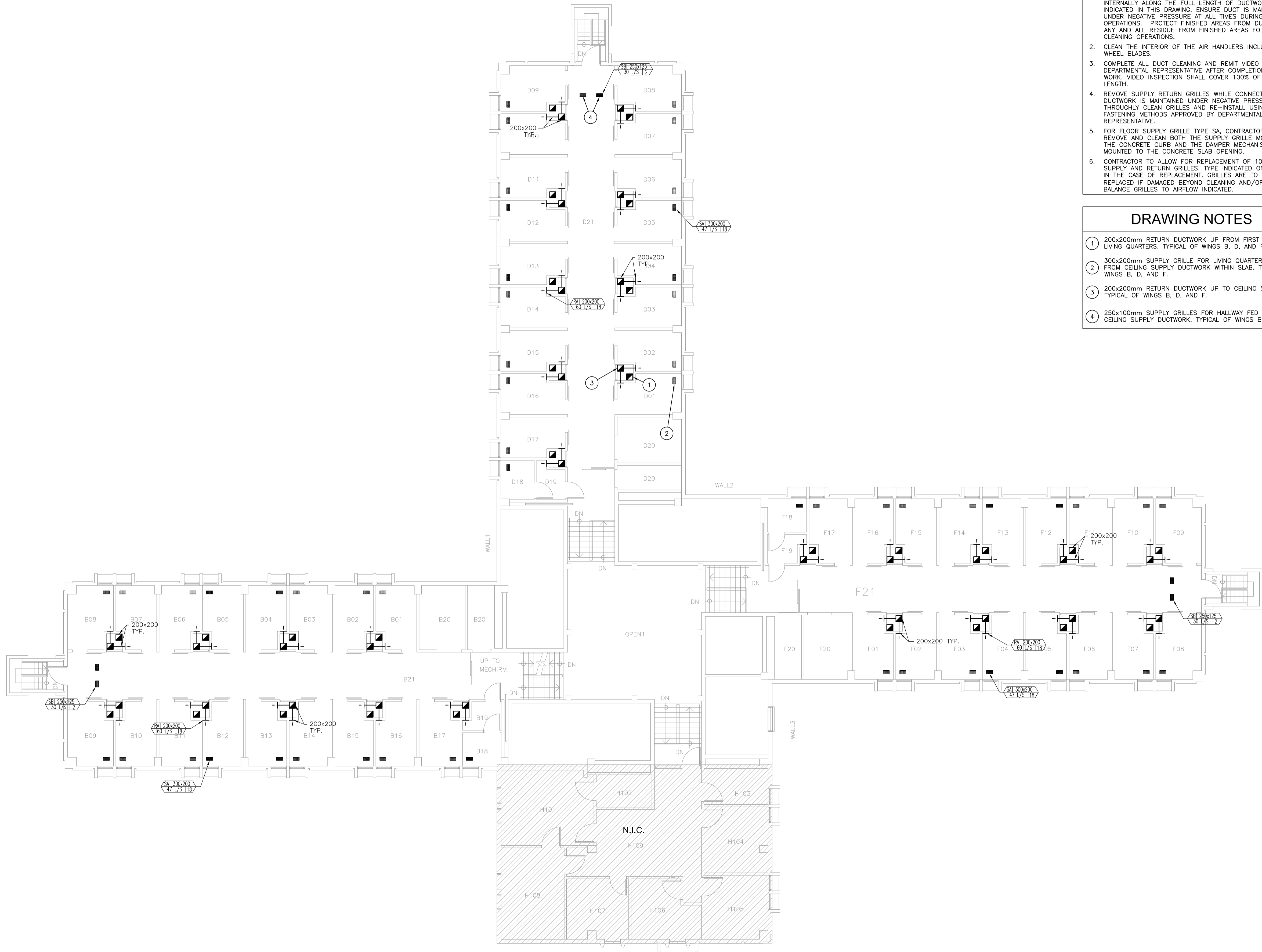
1 FLOOR 2 EXISTING HVAC LAYOUT SCALE: 1:100
