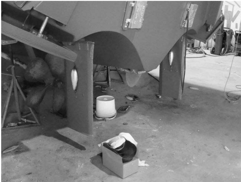
Figure H-06-2 Rudder – with view of rudder stock
