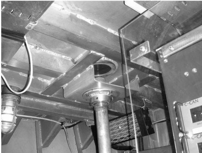
Figure H-06-1 Extended spindle for emergency steering
