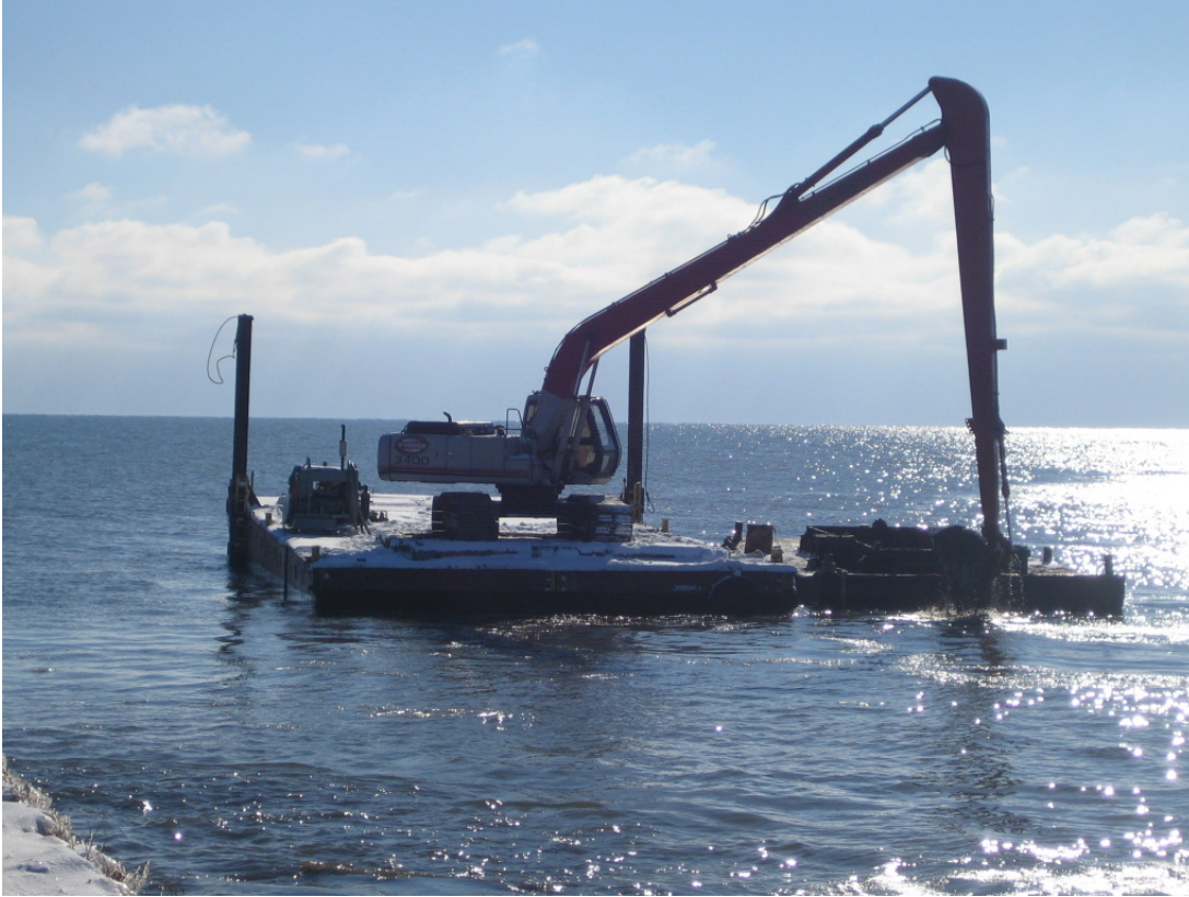
Figure 2.5 Backhoe, Spud Barge and Dump Scow, December 2005
