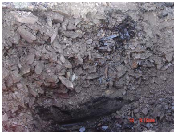
Photo 9 : Tar found in fill material at 02-TP06-04.
