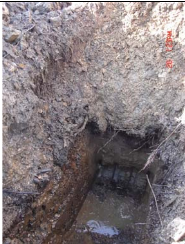
Photo 23 : Presence of water coming from the fill material layer at surface. 08-TP06-03
