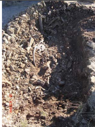
Photo 12 : Bedrock outcrop at 0.4m below ground surface at 02-TP06-12. Steel pipe fixture anchored in bedrock.
