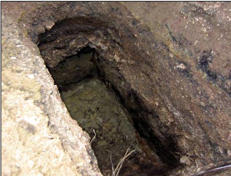
Photo 3.4: TP11, exceedences of PHC fractions and BTEX at depths up to 3m bgs.
