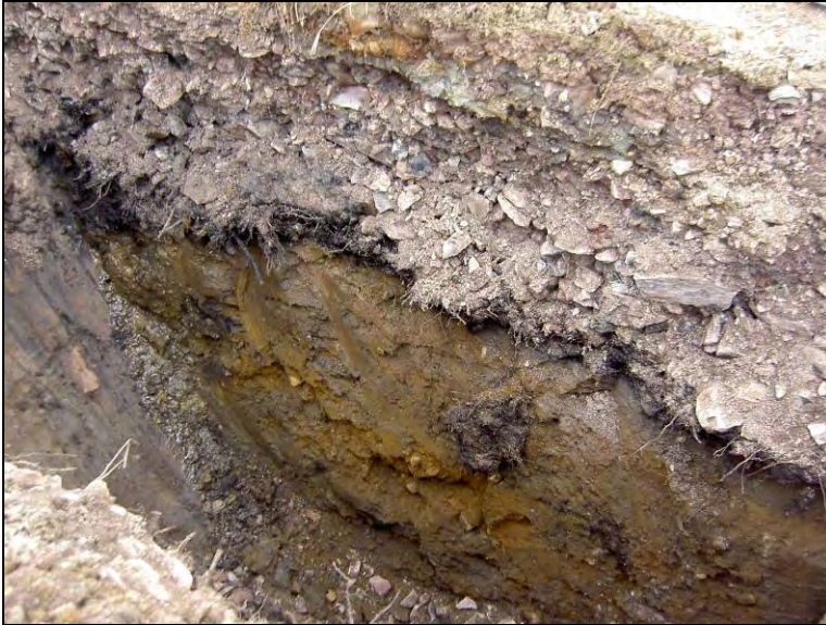
Photo 3.2: Native peat and silt, overlain by crushed shale fill. Minor seepage noted in left corner (TP05).
