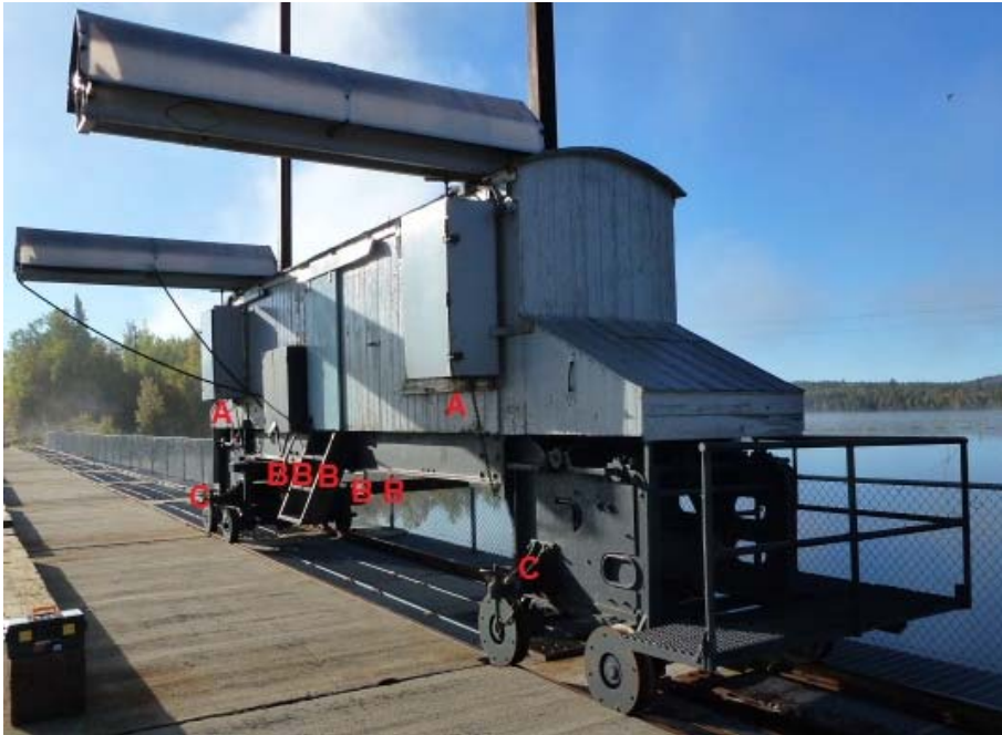
Figure 1 - Stoplog lifter looking upstream. "A" denotes approximate location of new personnel anchorages. "B" denotes approximate locations of beams on undercarriage which require end support brackets. "C" denotes devices on stoplog lifter that engage with deck anchors.
