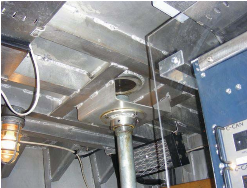
Figure HD-06-Fig. 1 Extended spindle for emergency steering.
