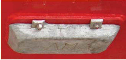
Figure HD-04-Fig. 1 - 10 Kg Zinc Hull /Transom anode
