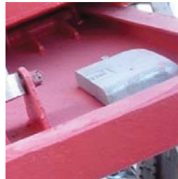
Figure HD-04-Fig. 3 – Rudder/Trim Tab Anodes
