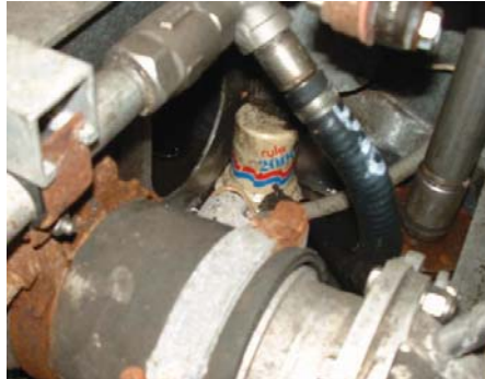
HD-05-Fig. 3&F4 – Engine Room Submersible Pumps (Port Left, Stbd Right)
