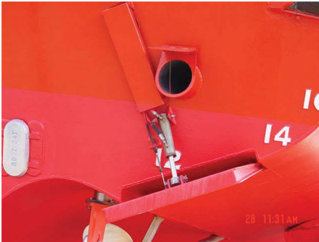
Figure HD-08-Fig. 1 Trim tab starboard side
