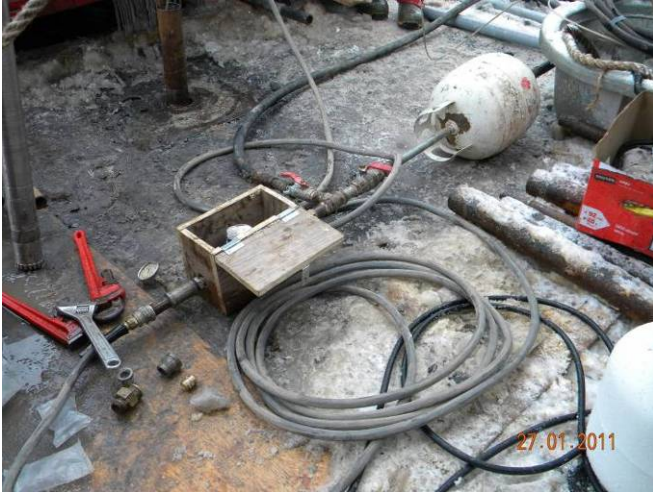
Water Pressure Testing - 3
