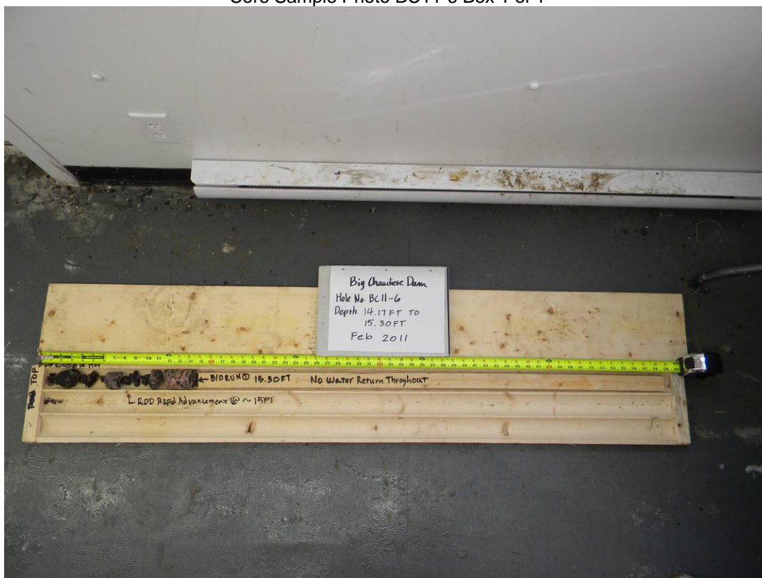
Core Sample Photo BC11-7 Box 1 of 1
