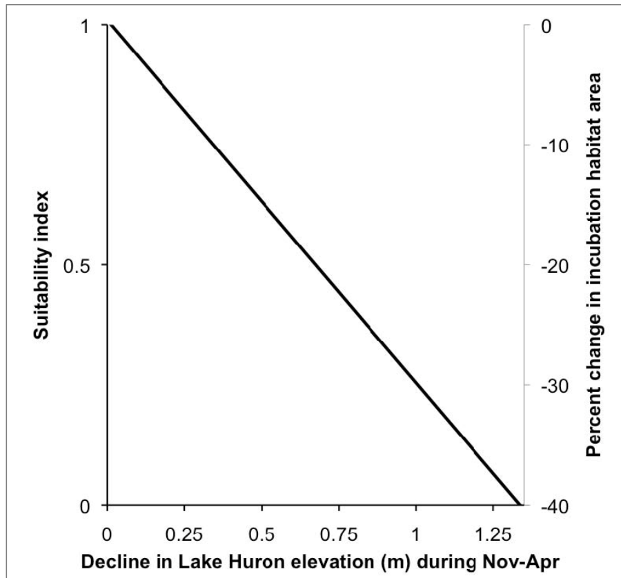
Figure 1. Relationship between Lake Huron water elevation and the percent change in cisco habitat area to determine a suitability index value.
