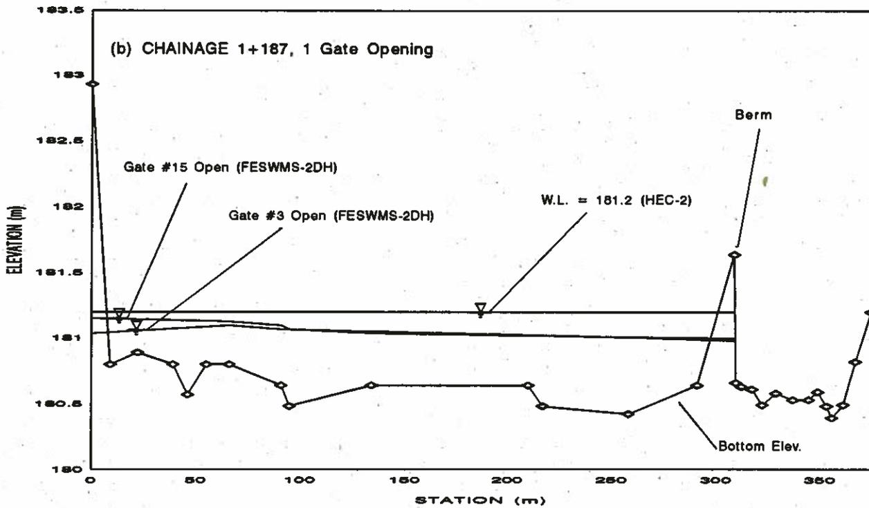
FIGURE 5.11 CROSS SECTION AT CHAINAGE 1+187 (1/2 and 1 GATES FLOW RATES)
