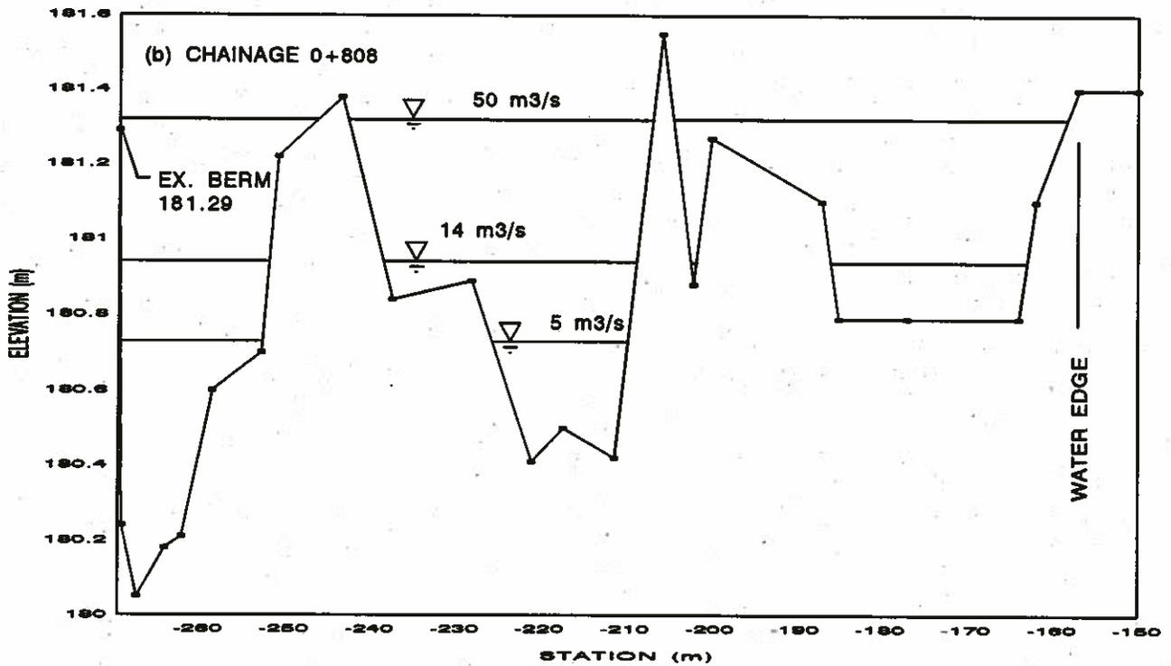
FIGURE 4.3 CROSS SECTION OF RAPIDS, NORTH OF BERM
