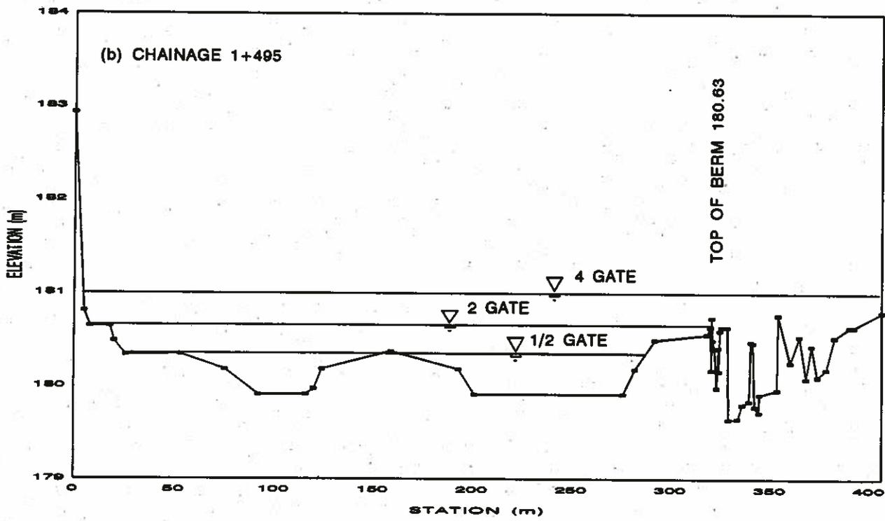
FIGURE 5.3 CROSS SECTION OF RAPIDS, SOUTH OF BERM
