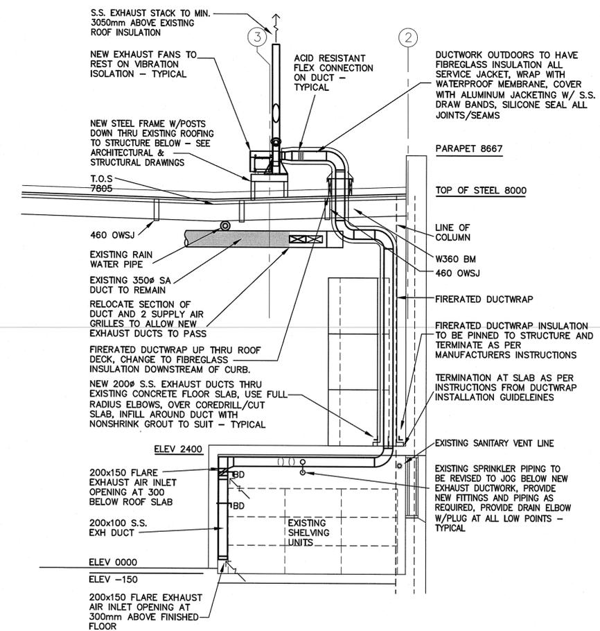
3 SECTION - EXHAUST DUCT WORK LOOKING WEST
