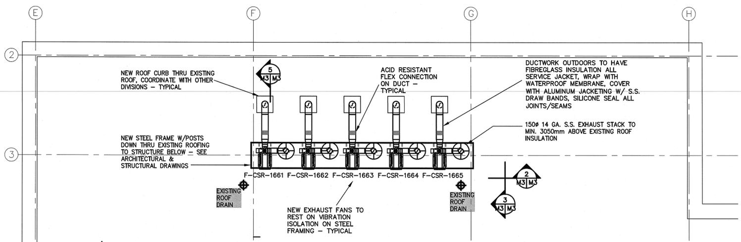
1 PARTIAL ROOF PLAN - VENTILATION - NEW
