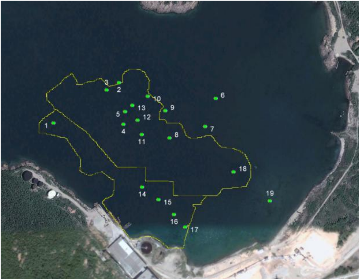
Figure 4: Sediment Grab Sampling Stations from 2012 (GPS locations are presented in Table 1)
