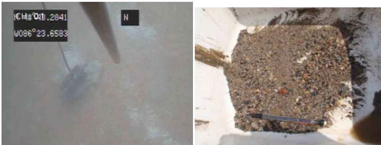
Figure 4. Petite ponar grab in action (left) and medium sand ponar grab sample (right).
