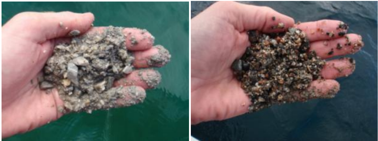
Figure 5. Coarse (Ponar # 17, left) and medium (Ponar # 2, right) sand capping material.
