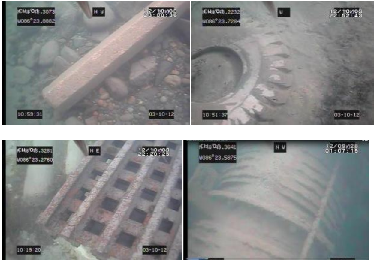
Figure 26. Industrial debris and large water intake pipe observed in or near cap zone.
