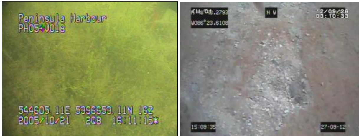
Figure 20. Dense stonewort along southern edge of cap zone in 2005 and at the same location ( \pm 2 m) in Sept 2012 after the application of coarse capping material.
