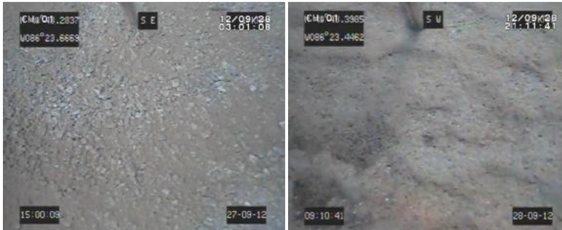
Figure 7. Coarse sand used for capping (left) and uncapped silt (right).
