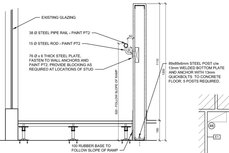
3 SECTION THROUGH RAMP SCALE 1:10
