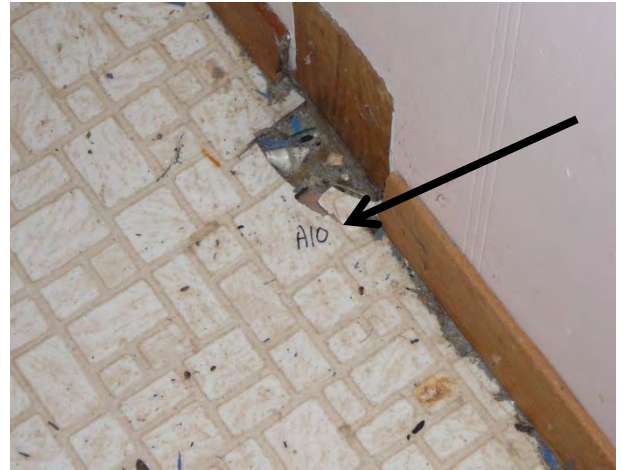
Sample A10 : Linoleum containing asbestos on laundry room floor
