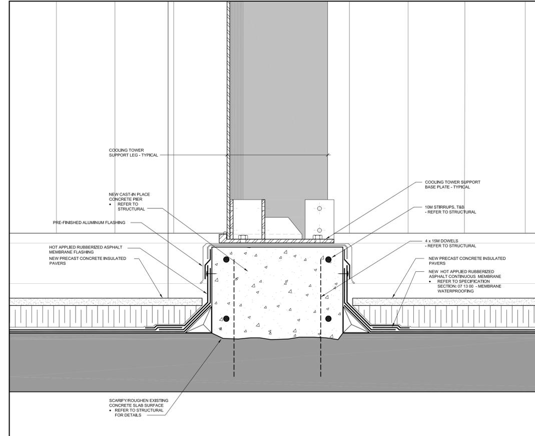
02 TYPICAL NEW SUPPORTING PIER SECTION DETAIL
