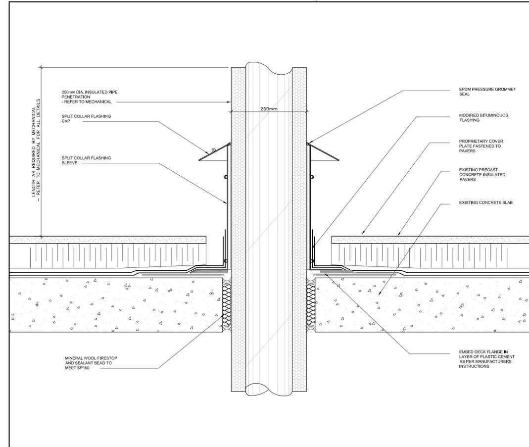
05 SECTION DETAIL AT INSULATED PIPE PENETRATION THROUGH ROOF
