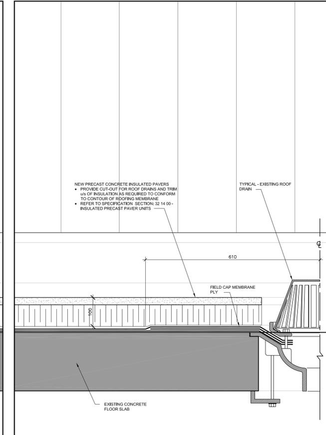
01 TYPICAL ROOF SECTION DETAIL AT FLOOR DRAIN
