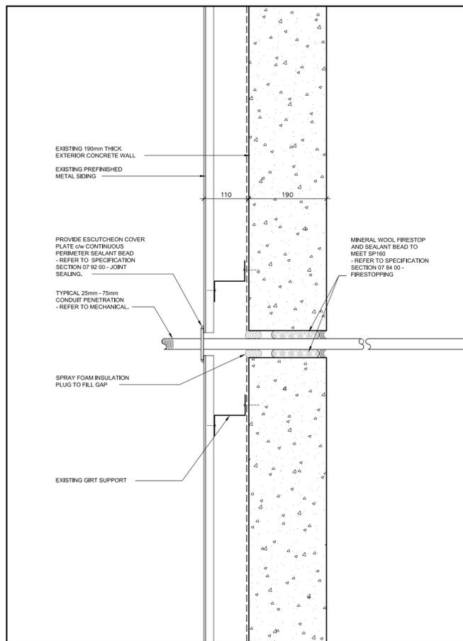
04 TYPICAL CONDUIT PENETRATION SECTION DETAIL
