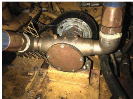
HD-05-Fig. 1 – Fire Pump looking aft
