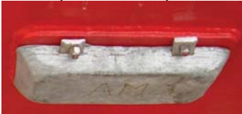
Figure HD-04-Fig. 1 - 10 Kg Zinc Hull /Transom anode
