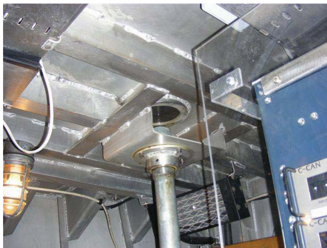
Figure HD-06-Fig. 1 Extended spindle for emergency steering.
