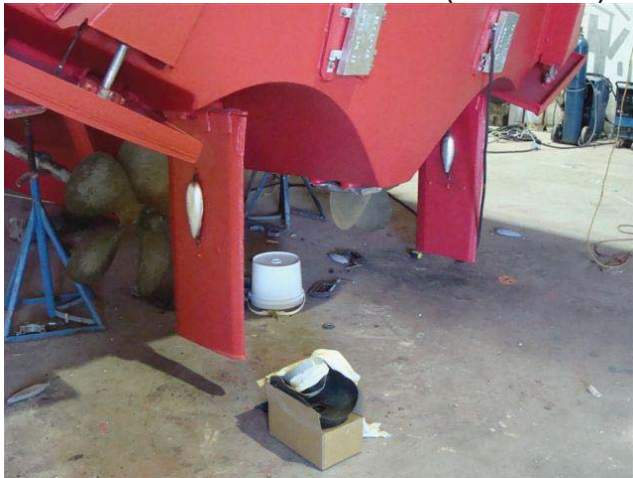
Figure HD-06-Fig. 2 Rudders with view of rudder stocks.
