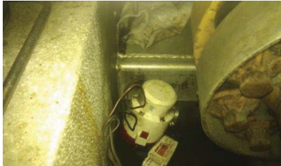
HD-05-Fig. 3&F4 – Engine Room Submersible Pumps (Port Left, Stbd Right)
