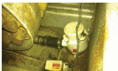
HD-05-Fig. 3&F4 – Engine Room Submersible Pumps (Port Left, Stbd Right)
