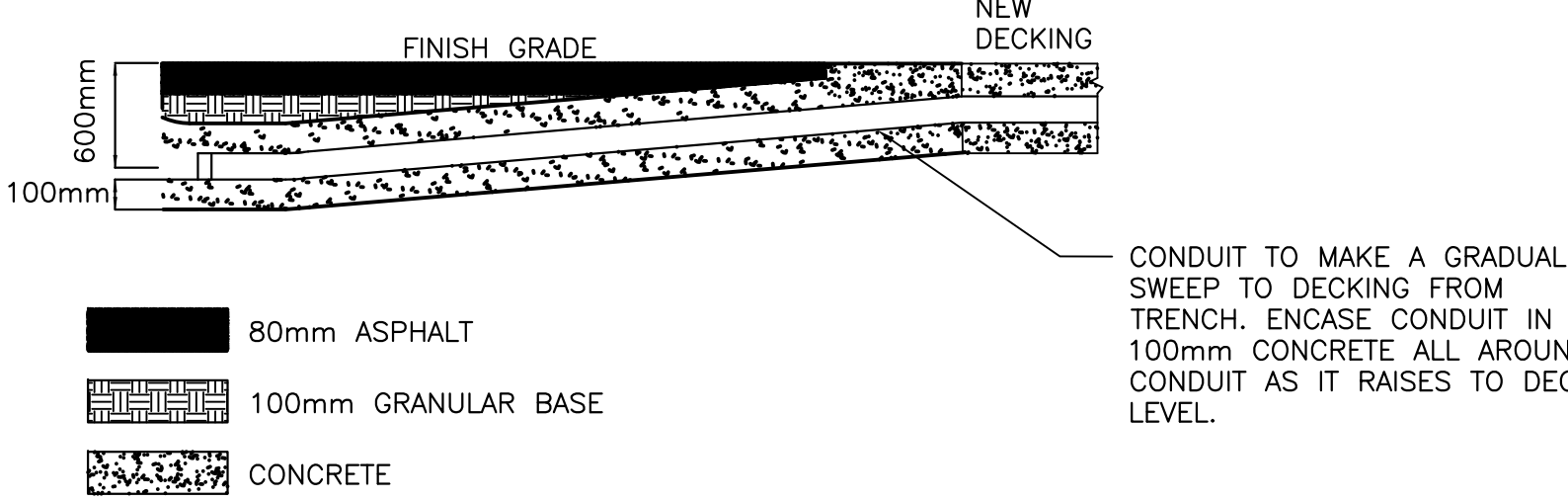
GRADUAL SLOPE FROM TRENCH TO DECKING J N.T.S. E2 E4
