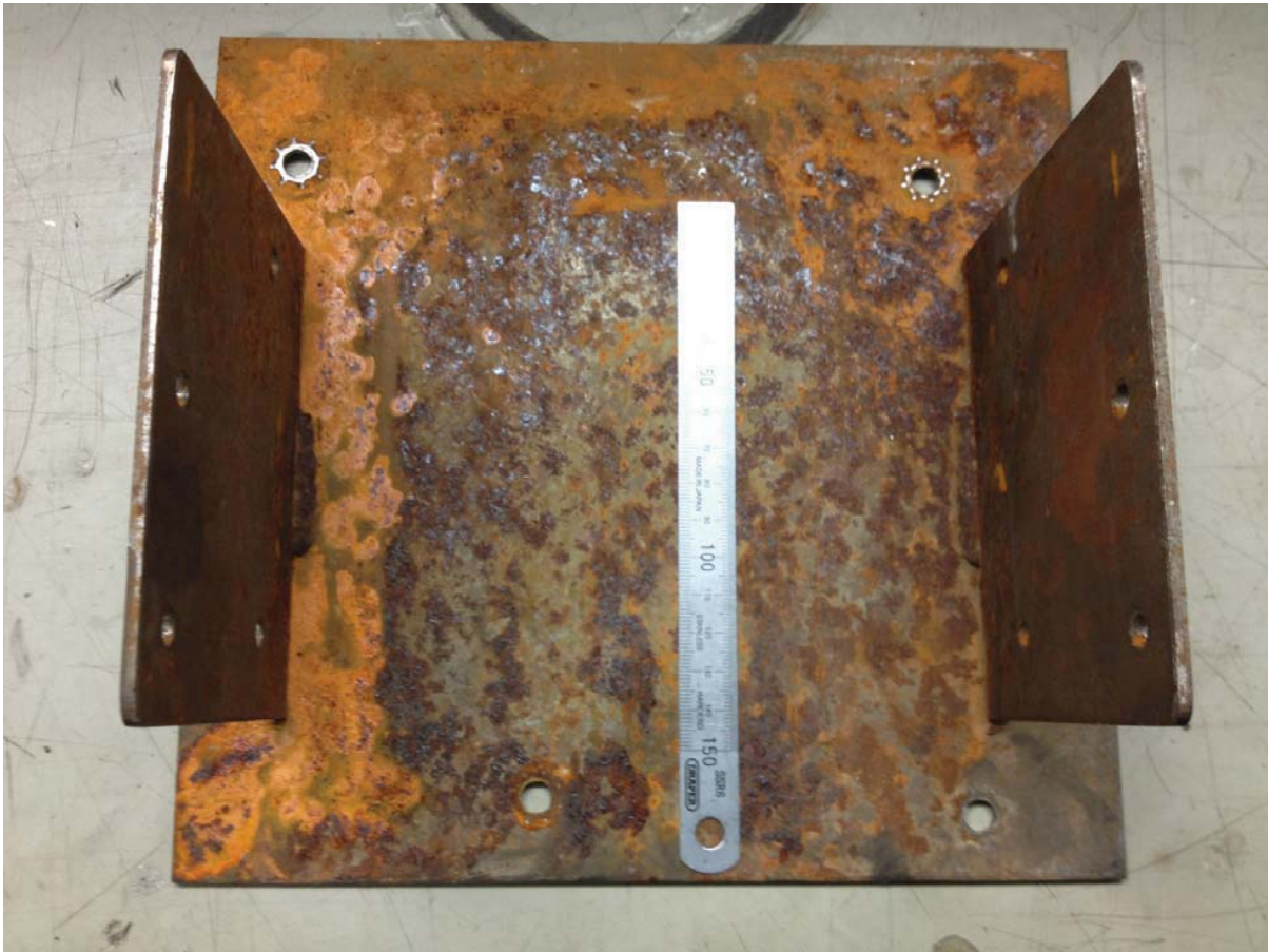
Photo #7 BSN Radio Mount. Made of aluminum.
