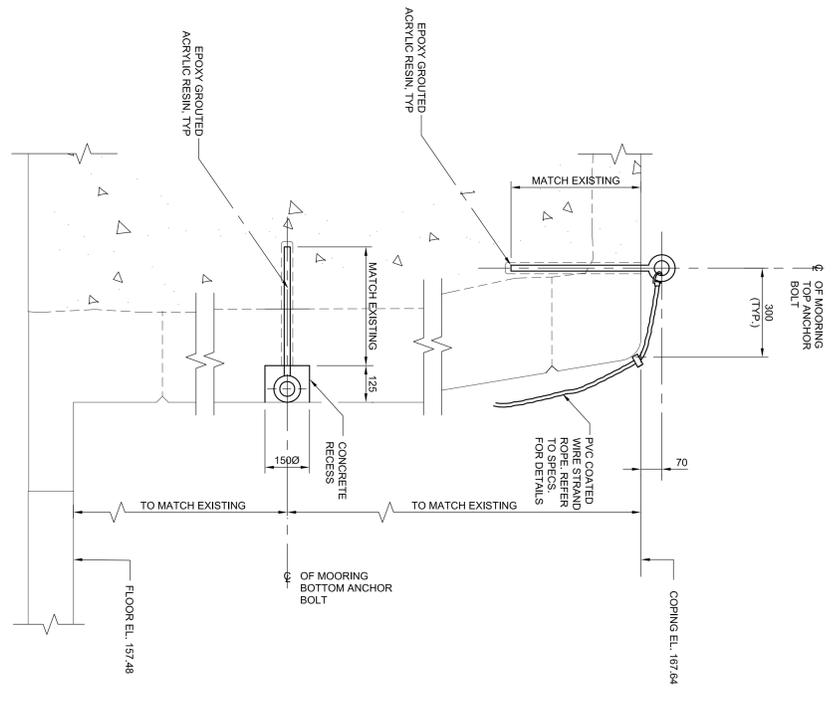
**MOORING CABLE ANCHORAGE - DETAIL**
