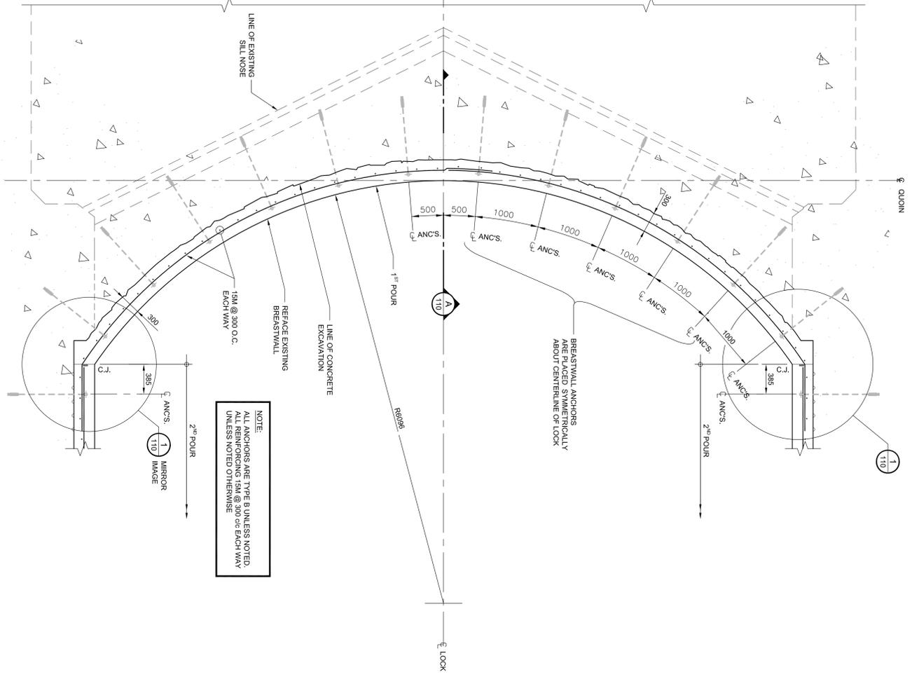
**BREASTWALL CONCRETE REPAIRS - HORIZONTAL SECTION**
