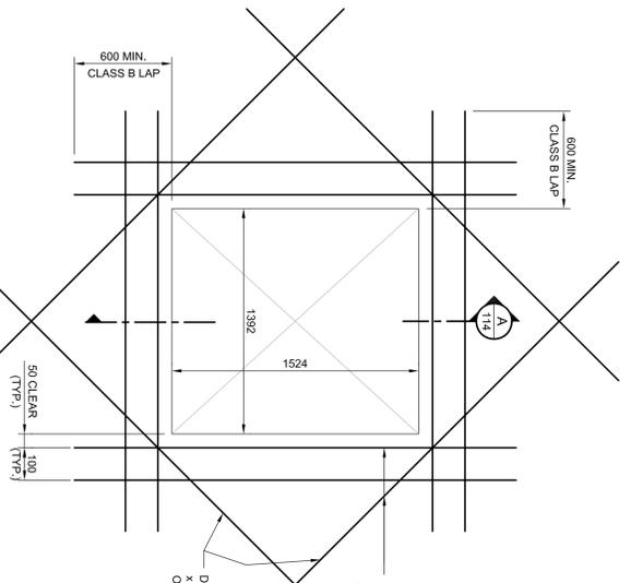
**PUSH BAR TUNNEL WALL OPENING - DETAIL**
