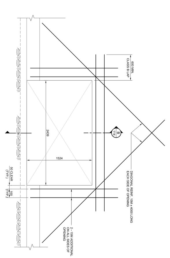
**DISCHARGE CULVERT WALL OPENING - DETAIL**
