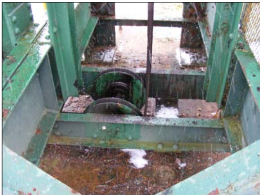
37 H16 COUNTERWEIGHT GUIDE CABLE AND SHEAVES
