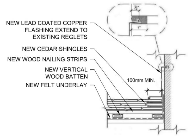
6 CHIMNEY FLASHING DETAIL
