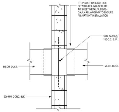
1 TYPICAL SECTION -DUCT SECURITY BARS
