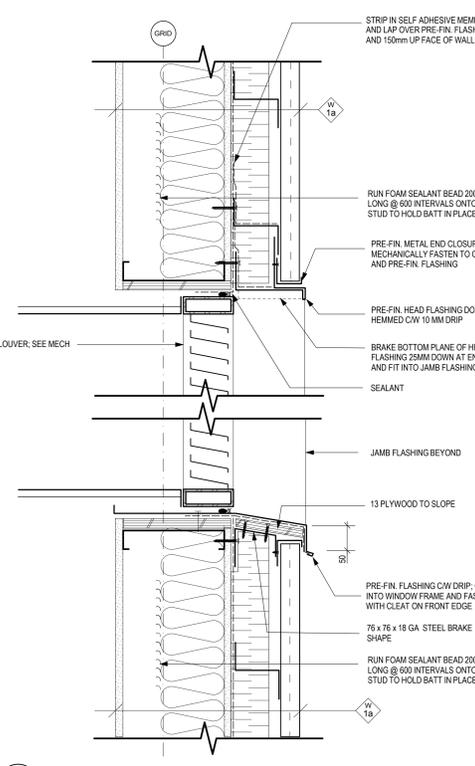
Q TYP. STUD WALL MECH. LOUVER SECTION
