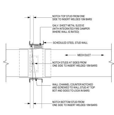
3 TYPICAL SECTION -DUCT SECURITY BARS AT STUD WALL
