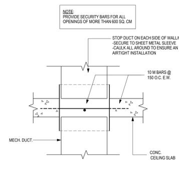
2 TYPICAL SECTION -DUCT SECURITY BARS AT CONCRETE SLAB
