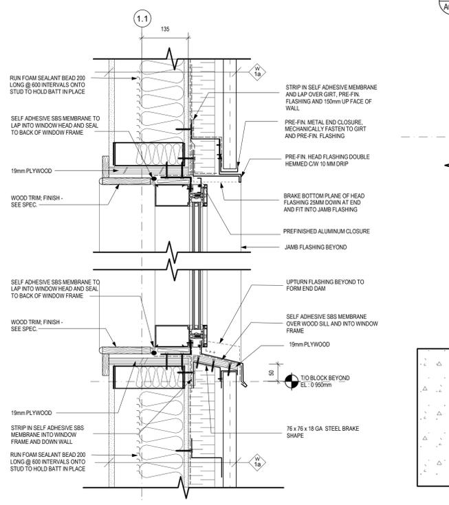
**Q TYPICAL STUD WALL AT MAIN FLOOR**
