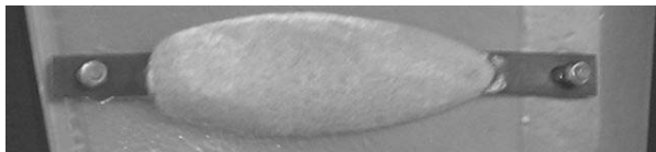
Figure HD-04-3 Rudder anode
