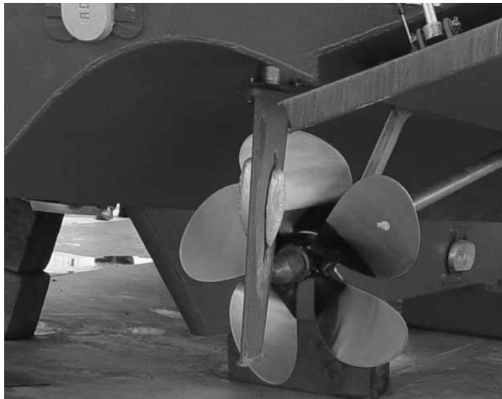
Figure H-03-1 Rudder – with view of rudder stock
