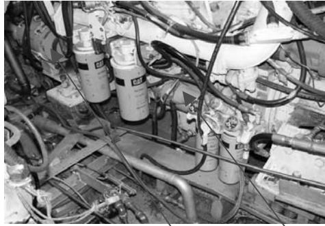
Figure L-01-1 Starboard alternator and starter
