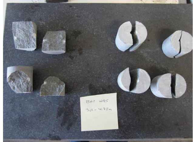
Photo 30 – Point load testing – BH3 NQ5, 3.2 to 4.72 m
