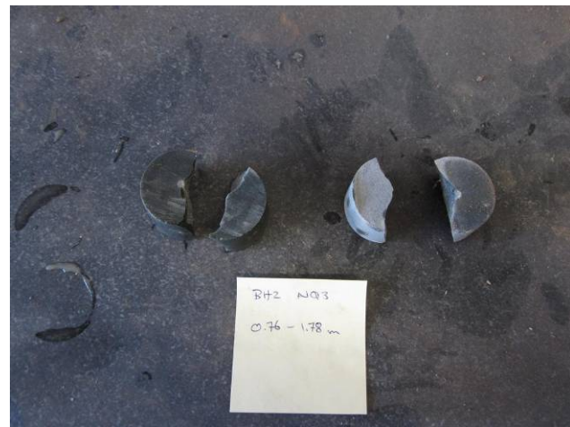
Photo 26 – Point load testing – BH2 NQ3, 0.76 to 1.78 m
