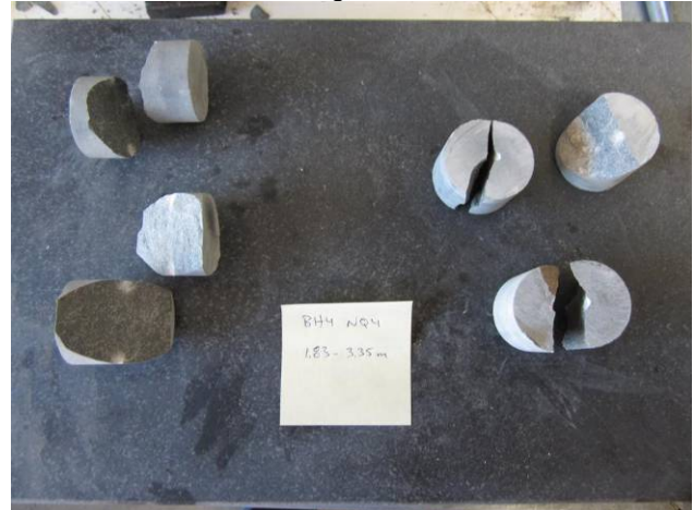
Photo 32 – Point load testing – BH4 NQ4, 1.83 to 3.35 m
