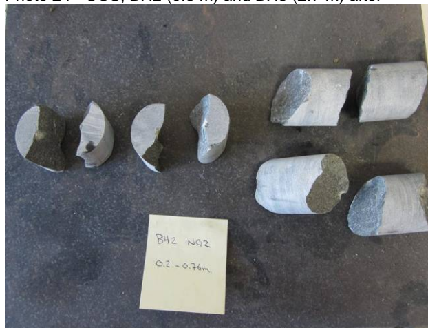
Photo 25 – Point load testing – BH2 NQ2, 0.2 to 0.76 m
