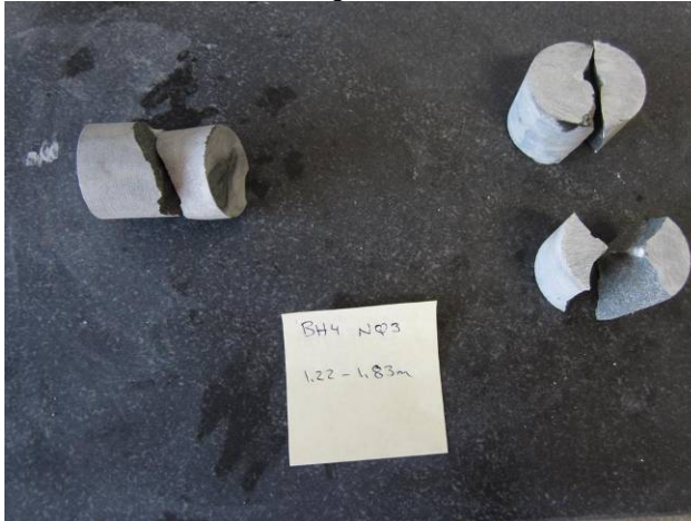
Photo 31 – Point load testing – BH4 NQ3, 1.22 to 1.83 m
