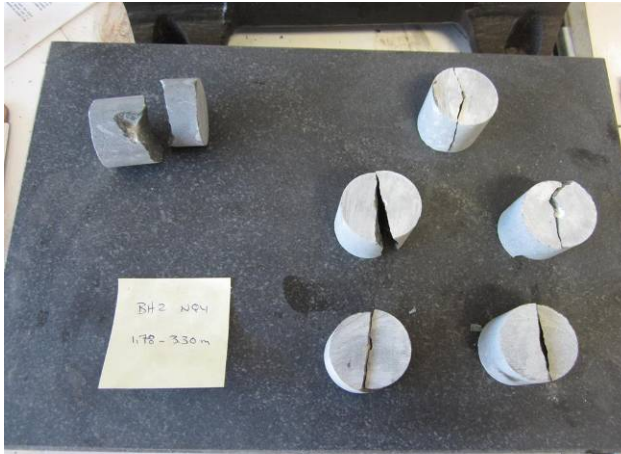
Photo 27 – Point load testing – BH2 NQ4, 1.78 to 3.30 m
