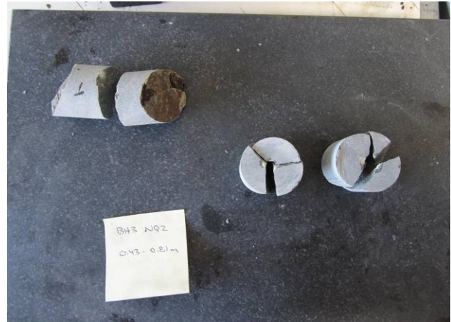
Photo 28 – Point load testing – BH3 NQ2, 0.43 to 0.81 m
