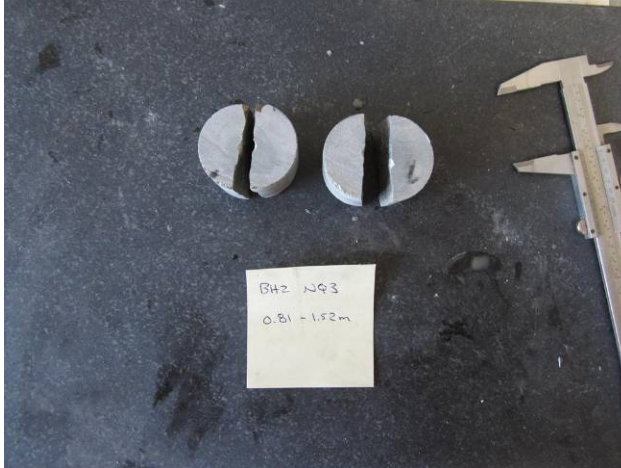
Photo 29 – Point load testing – BH3 NQ3, 0.81 to 1.52 m
