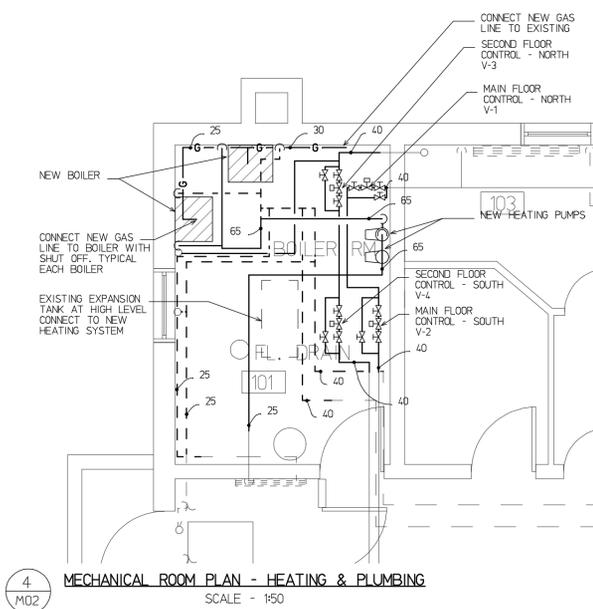
4 MECHANICAL ROOM PLAN - HEATING & PLUMBING
