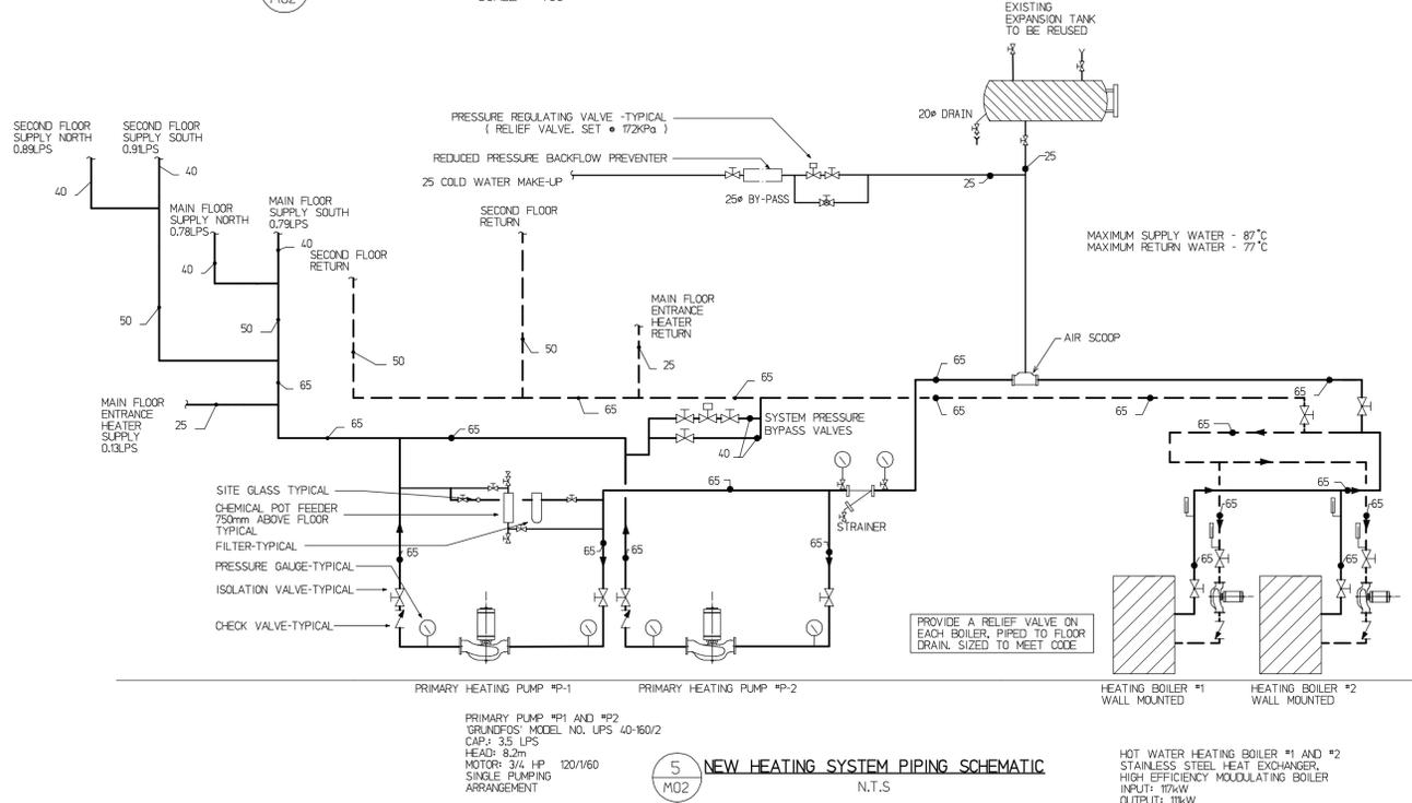
5 NEW HEATING SYSTEM PIPING SCHEMATIC
