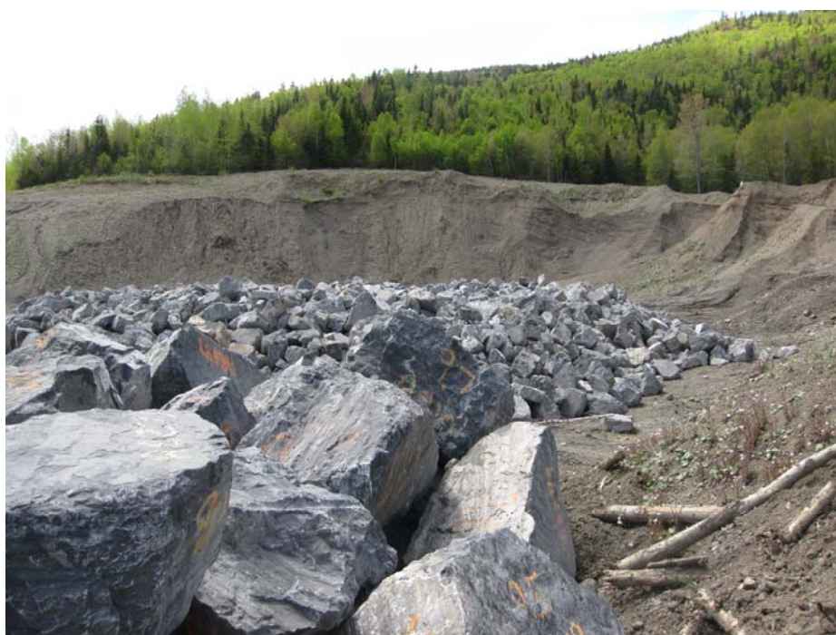
Photo 10 - Stone size 8-12 mt and 100 and 300 kg provided by PWGSC. They are located in Allen Dumaresq's career at Rivière-au-Renard.
